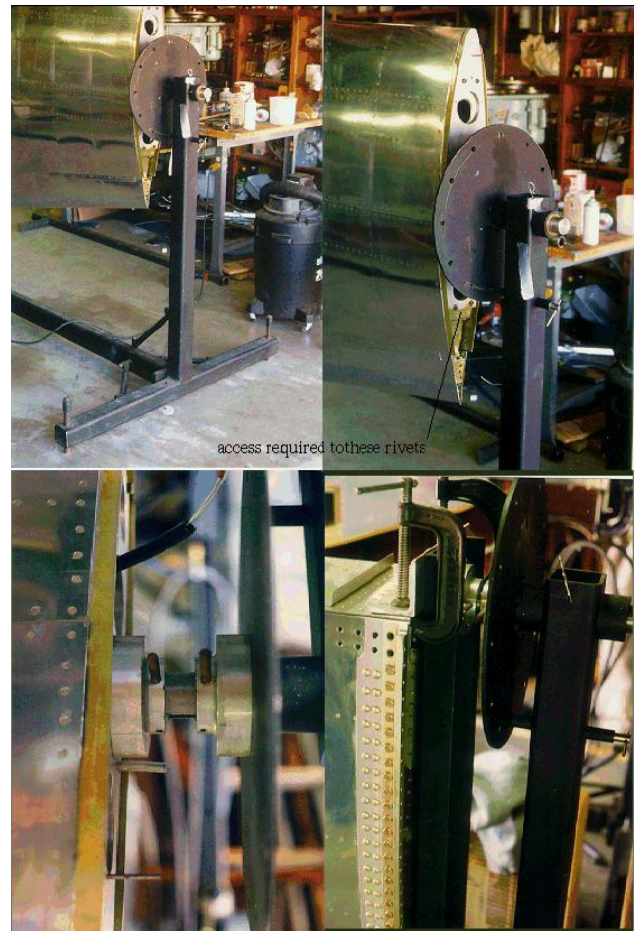
Figure 1.1. An example of a wing assembly fixture. This one has index plates on both ends so that the wash-out is preserved upon rotation.
