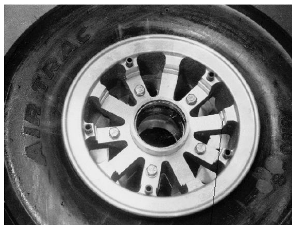
You must trim either the inboard wheel half or the outboard caliper
