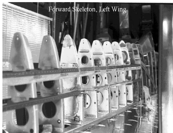
Figure 1.7. View of the ribs and stringers in the left wing forward of the main spar.
