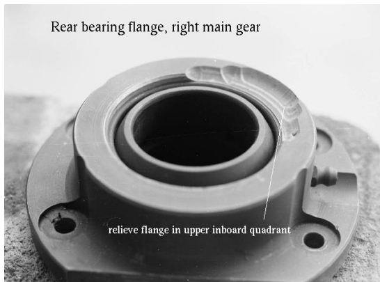
Figure 1.11. You will have to relieve the rear bearing flange in the upper inboard quadrant in order to get the trunion to seat properly.
