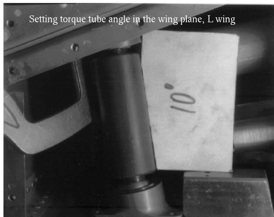
Figure 1.38. View of the torque tube in the left wing from the bottom. The leading edge is up, so the rear bearing is at the bottom.
