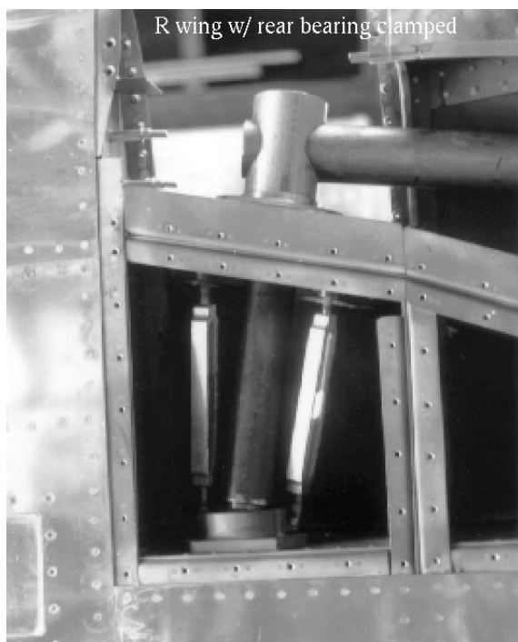
Figure 1.27. Clamps made from turnbuckles can be used to hold the rear bearing in place during alignment.
