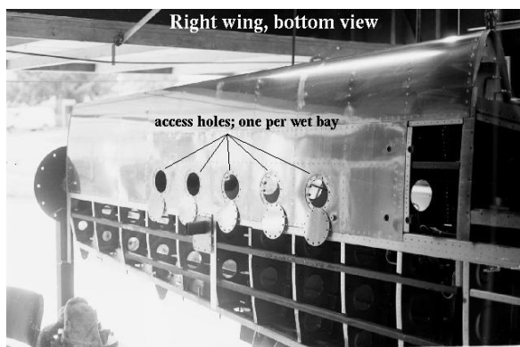
Figure 1.9. You need to put an access plate in each bay of the wet part of the wing (or else you better have very small hands attached to long, rubber arms!)
