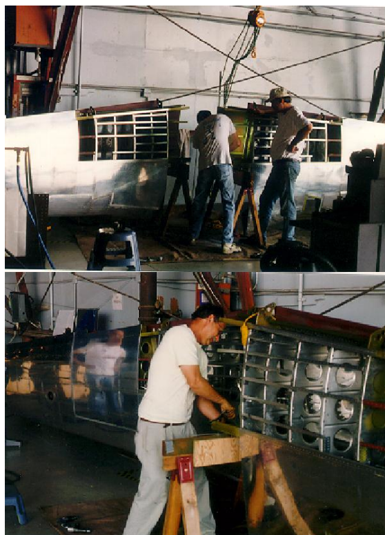
Figure 1.19. Preparing to mate the wings.
