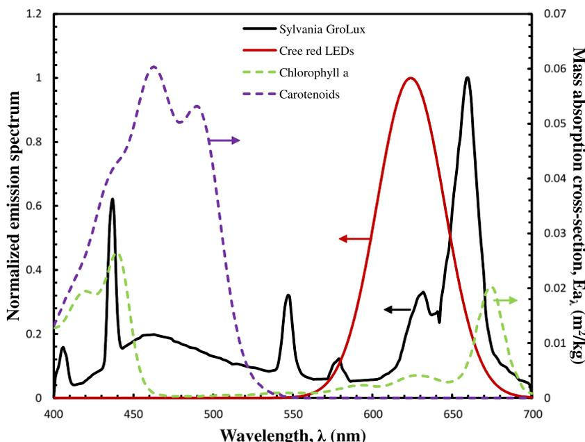
**Fig. 1.** Normalized emission spectrum of Sylvania GroLux white fluorescent light source and Cree red LEDs used for *N. oculata* cultivation along with *in vivo* absorption cross-sections (in m<sup>2</sup>/mg) of chlorophyll *a*, carotenoids (Bidigare et al., 1990). (For interpretation of the references to color in this figure legend, the reader is referred to the web version of this article.)
