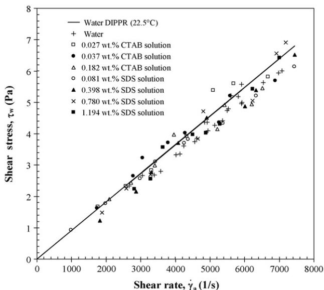
Fig. 1. Shear stress versus shear rate measured for deionized water and aqueous solutions of SDS and CTAB at various concentrations.
