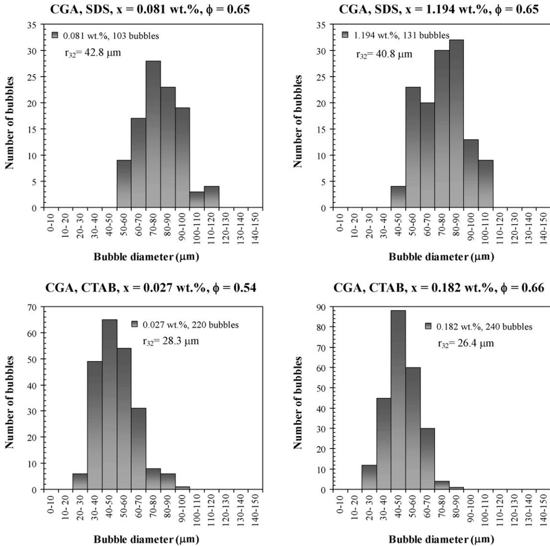
Fig. 3. Bubble size distribution of CGA formed with different SDS and CTAB aqueous solutions at  $25 \pm 2^\circ\text{C}$  corresponding to micrographs shown in Fig. 2.
