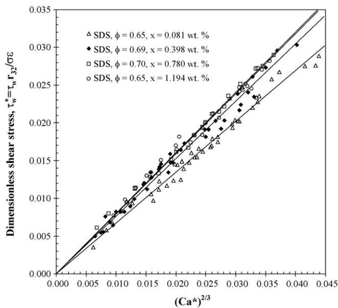
Fig. 7. Dimensionless volume equalized wall shear stress  $\tau_w^*$  versus  $(Ca^*)^{2/3}$  for CGA made from SDS aqueous solution with different concentrations.
