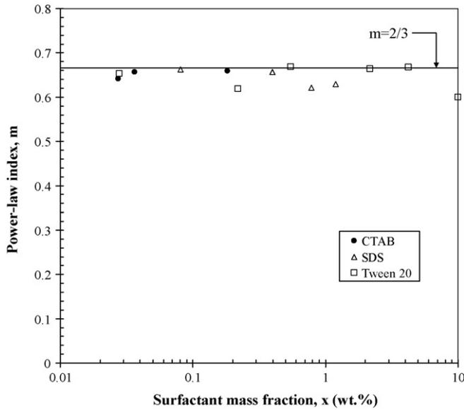
Fig. 6. Empirical power-law index  $m$  as a function of surfactant mass fraction  $x$  obtained in the 1.5 mm diameter pipe at  $25 \pm 2^\circ\text{C}$  for microfoams made of SDS, CTAB, and Tween 20. Solid line corresponds to  $m=2/3$ .
