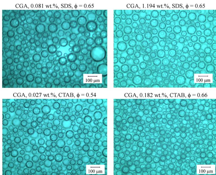
Fig. 2. Typical micrograph of CGA formed with different aqueous solutions of SDS (top) and CTAB (bottom) at 25 ± 2 °C.
