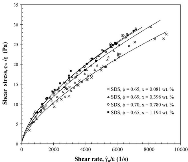
Fig. 4. Volume equalized shear stress versus shear rate for CGA made from SDS aqueous solution with different concentrations obtained in the 1.5 mm diameter pipe at  $25 \pm 2^\circ\text{C}$ .
