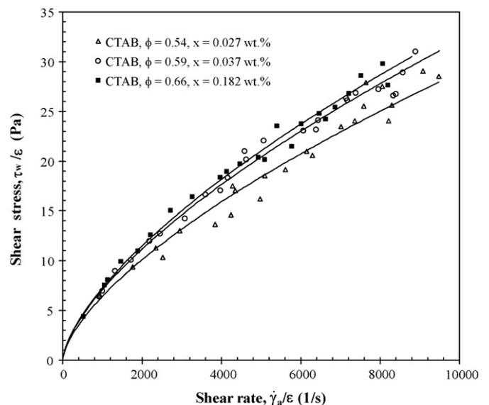
Fig. 5. Volume equalized shear stress versus shear rate for CGA made from CTAB aqueous solution with different concentrations obtained in the 1.5 mm diameter pipe at  $25 \pm 2^\circ\text{C}$ .
