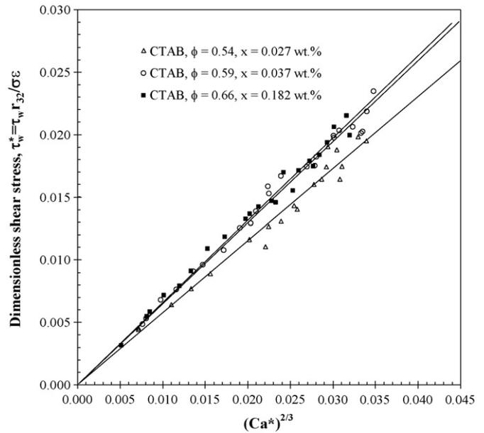
Fig. 8. Dimensionless volume equalized wall shear stress  $\tau_w^*$  versus  $(Ca^*)^{2/3}$  for CGA made from CTAB aqueous solution with different concentrations.
