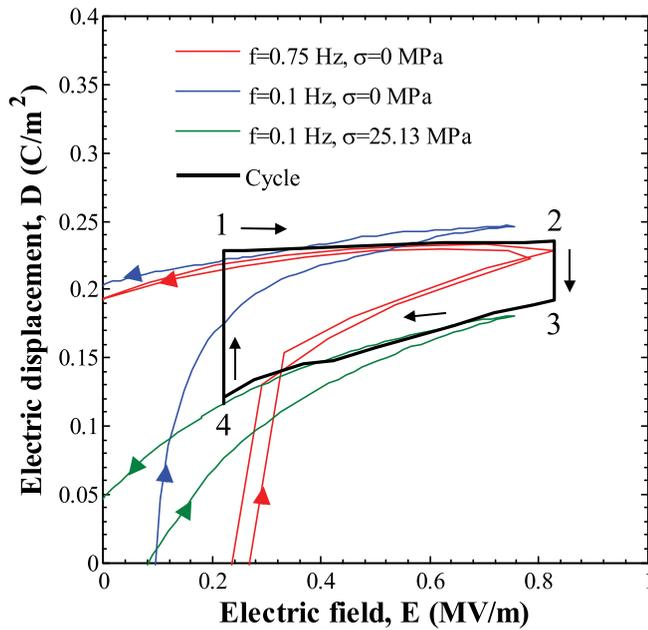
FIG. 5. Isothermal bipolar  $D$ - $E$  loops collected at 0.1 or 0.75 Hz and experimental power cycle performed at frequency  $f = 1$  Hz on PMN-28PT for electric field between  $E_L = 0.2$  MV/m and  $E_H = 0.8$  MV/m at  $T_b = 80^\circ\text{C}$  and compressive stress between  $\sigma = 0$  and  $\sigma_H = 25.13$  MPa. The power cycle was vertically displaced to match the  $D$ - $E$  loop at  $T = 80^\circ\text{C}$  and  $\sigma_H = 25.13$  MPa.
