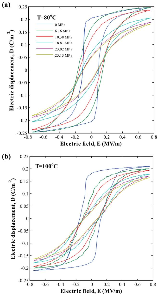
FIG. 3. Isothermal bipolar  $D$ - $E$  loops of [001] PMN-28PT at 0.1 Hz for temperatures (a)  $80^\circ\text{C}$  and (b)  $100^\circ\text{C}$  and compressive stress  $\sigma$  between 0 and 25.13 MPa.
