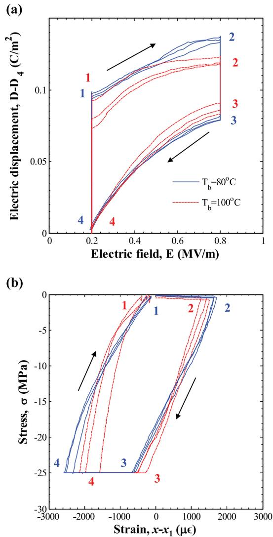
FIG. 8. (a) Experimentally measured stress versus strain diagrams for the thermally biased mechanical power cycle performed at  $T_b = 80^\circ\text{C}$  and  $100^\circ\text{C}$ . (b) Experimentally measured electric displacement versus electric field diagrams for the thermally biased mechanical power cycle performed  $T_b = 80^\circ\text{C}$  and  $100^\circ\text{C}$ . In all cases  $E_L = 0.2$  MV/m,  $E_H = 0.8$  MV/m, and  $\sigma_H = 25$  MPa.
