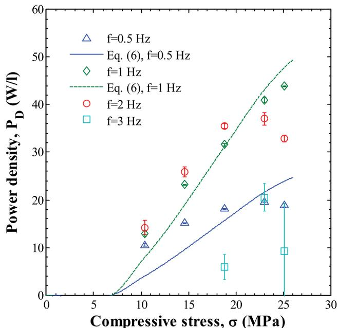
FIG. 7. Experimentally measured power density generated by performing the new power cycle on [001] PMN-28PT as a function of compressive stress  $\sigma_H$  for frequency ranging from 0.5 to 3 Hz. The bias-temperature  $T_b$  was maintained at 80 °C. The low and high electric fields  $E_L$  and  $E_H$  were set at 0.2 and 0.8 MV/m. The lines represent the predictions of the model given by Eq. (6) using properties retrieved from bipolar  $D$ - $E$  loops.
