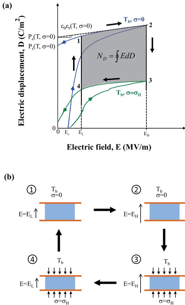
FIG. 1. (a) Two-dimensional projection of the new power cycle in the  $D$ - $E$  plane. Electric displacement versus electric field loops for uniaxial stress  $\sigma = 0$  and for  $\sigma_H$  at temperature  $T_b$ . The electrical energy generated per cycle is represented by the grey area enclosed between 1–2–3–4. (b) The thermal, electrical, and stress states of the ferroelectric sample during each point of the new power cycle.
