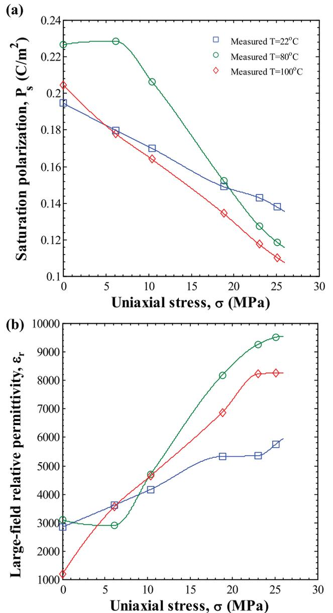
FIG. 4. (a) Saturation polarization  $P_s(T, \sigma)$  and (b) large-field relative permittivity  $\epsilon_r(T, \sigma)$  as a function of uniaxial stress retrieved from the isothermal bipolar  $D$ - $E$  loops of PMN-28PT at 0.1 Hz for temperatures 22, 80, and  $100^\circ\text{C}$  (Figure 3). The solid lines correspond to the piecewise cubic hermite interpolating polynomial fit.
