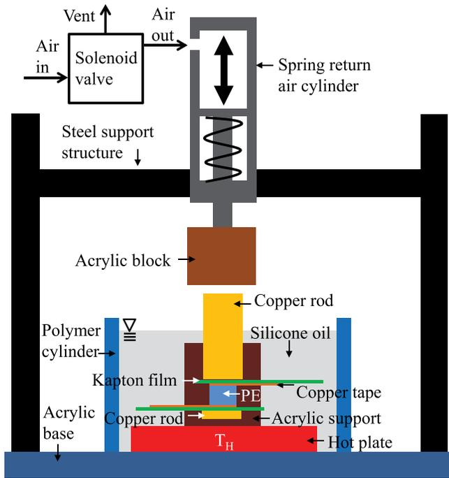
FIG. 2. Schematic of the thermomechanical subsystem used to create the temperature bias and to apply compressive stress during the new thermally biased mechanical power cycle depicted in Figure 1. Dimensions are not to scale.
