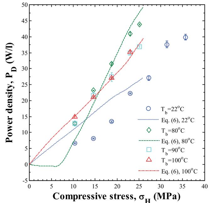
FIG. 6. Experimentally measured power density generated by performing the thermally biased mechanical power cycle on [001] PMN-28PT as a function of compressive stress. The bias-temperature  $T_b$  ranged from 22 to  $100^\circ\text{C}$ . The frequency was fixed at 1 Hz. The low and high electric fields  $E_L$  and  $E_H$  were set at 0.2 and 0.8 MV/m. The lines represent the predictions of the model given by Eq. (6) using properties retrieved from bipolar  $D$ - $E$  loops.
