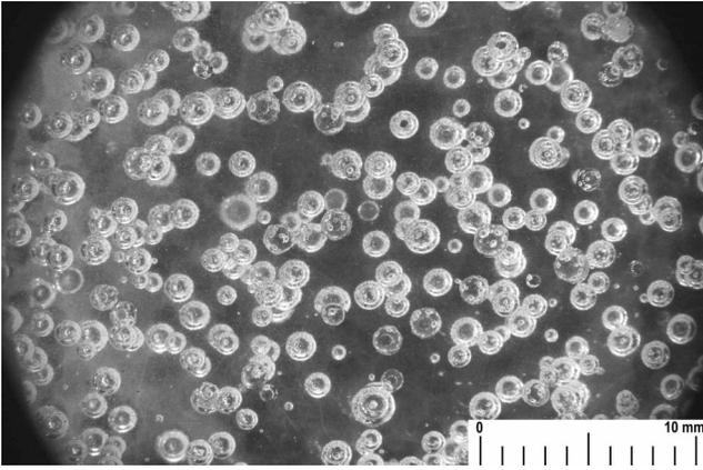
Fig. 3. Digital photograph of a 3-mm-thick fused quartz sample containing bubbles (porosity  $\approx 10\%$ ).
