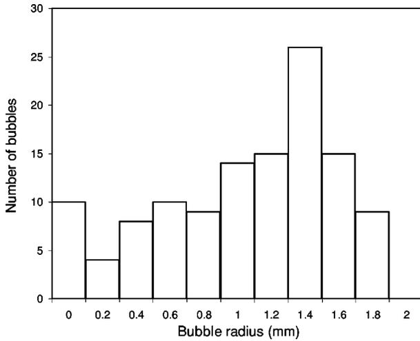
Fig. 4. Bubble size distribution obtained from more than 120 images of individual bubbles.
