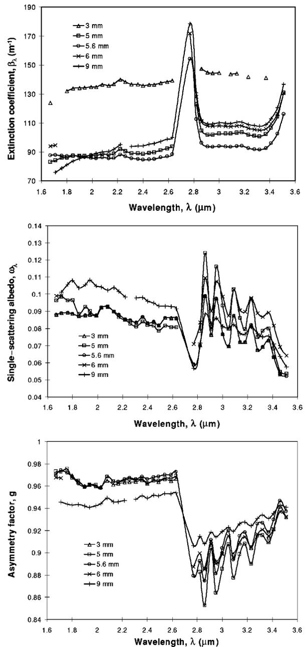
Fig. 7. Retrieved extinction coefficient, single-scattering albedo and Henyey-Greenstein asymmetry factor determined by an inverse method for each sample.
