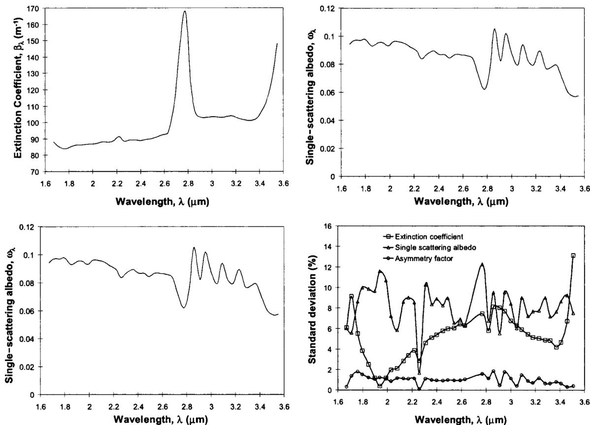
Fig. 8. Average retrieved extinction, single-scattering albedo, and Henyey–Greenstein asymmetry factor by an inverse method for each sample and their standard deviations.
