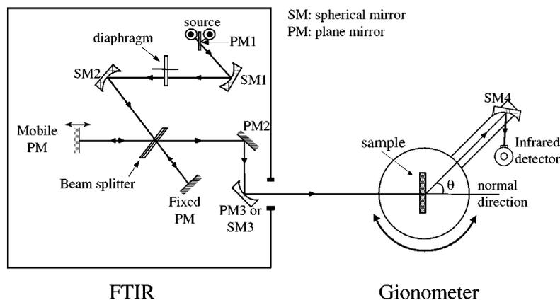
Fig. 1. Schematic of the experimental apparatus used to measure the spectral transmittance and reflectance.
