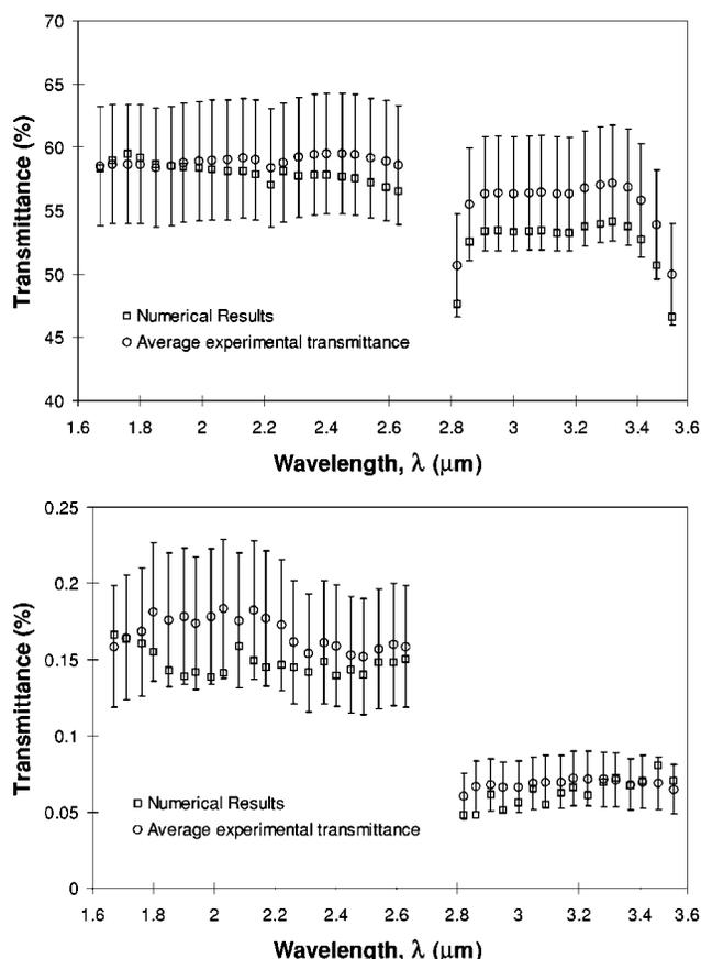
Fig. 10. Comparison between the average measured spectral transmittance with error bars corresponding to  $T_{e,\lambda}(\theta_i) \pm \Delta_i$  and the numerical results obtained with the averaged retrieved radiation characteristics for (top)  $\theta_i = 0^\circ$  and  $\Delta_i = 9\%$  and (bottom)  $\theta_i = 3.32^\circ$  and  $\Delta_i = 25\%$ .
