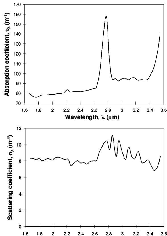
Fig. 9. Average retrieved absorption (top) and scattering (bottom) coefficients.
