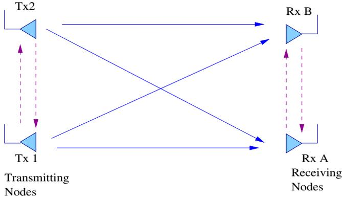
Fig. 2. Channel model for 4-node cooperation
