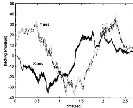
Fig. 4 Tracking errors for the MIMO controller
