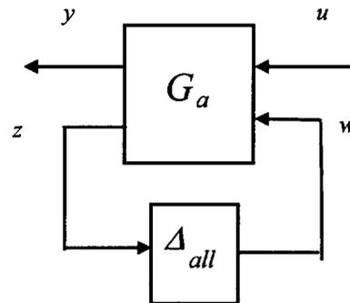
Fig. 2 Extended LFT representation for robust performance
