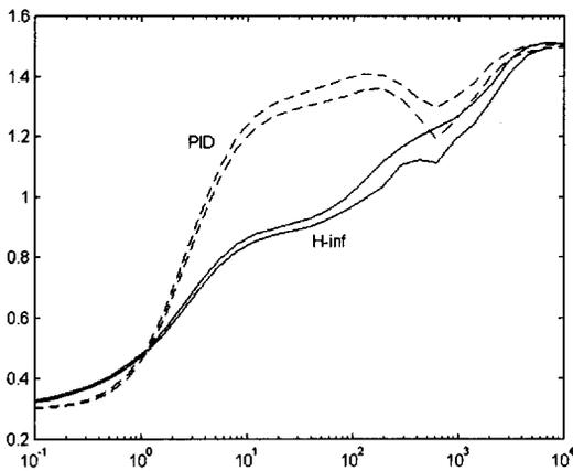
Fig. 3 Structured singular value for robust performance
