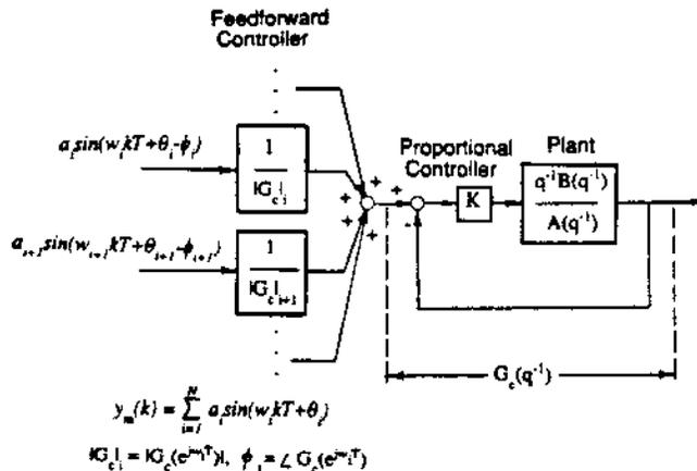
Fig. 6 Feedforward controller for tracking sinusoidal signals
