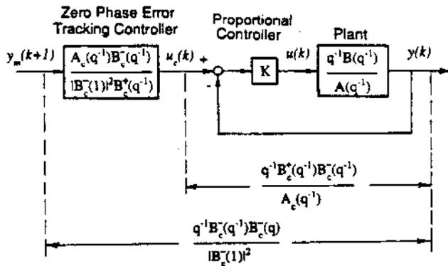
Fig. 7 Zero phase error tracking controller for tracking arbitrary signals
