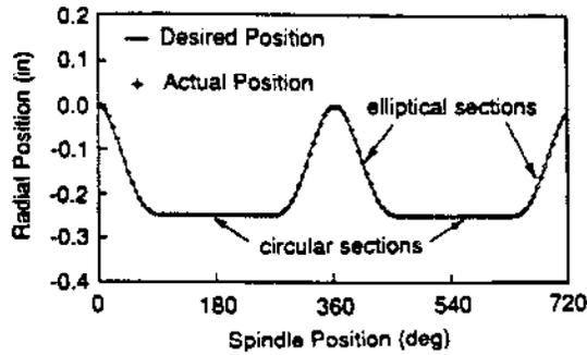
Fig. 10 Experimental result of noncircular cutting (cross-sectional shape = semicircle joined by semiellipses)
