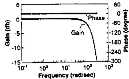
Fig. 8 Frequency response between desired output and actual output under zero phase error tracking control
