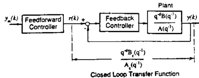
Fig. 3 Controlled plant under feedback/feedforward control
