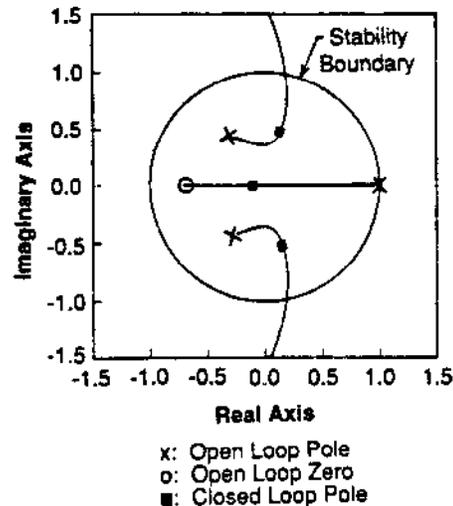
Fig. 4 Closed loop root locus for varying proportional feedback control gain  $K$
