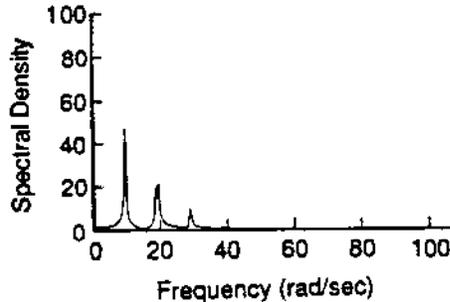
Fig. 11 Frequency spectrum of desired tool position (cross-sectional shape = semicircle joined by semiellipses)
