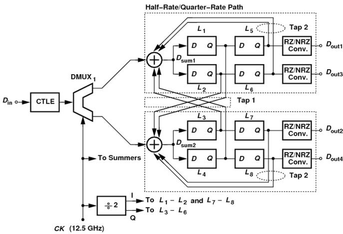
Figure 2.4.1: Equalizer architecture.
