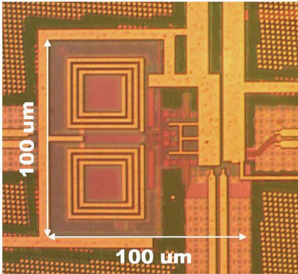
Figure 2.4.7: Equalizer die core in 45nm CMOS technology.
