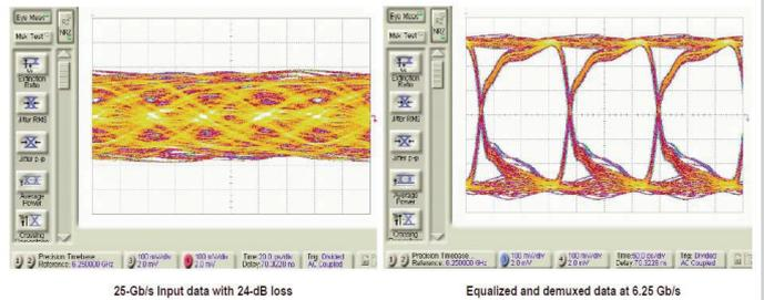
Figure 2.4.4: Measured eye diagrams of input and output data.
