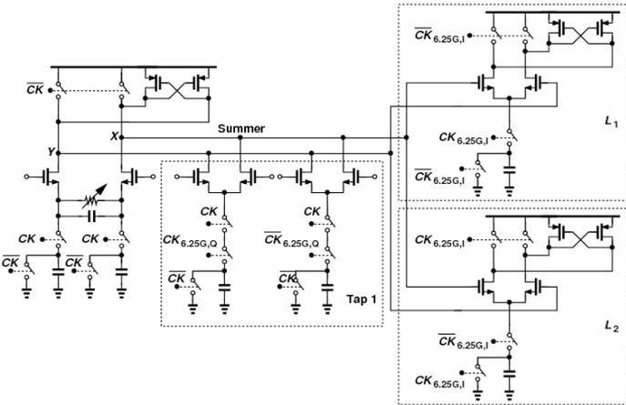
Figure 2.4.3: Implementation of one half-rate/quarter-rate path.
