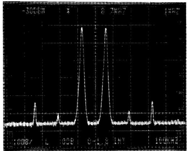
Figure 5: Output spectrum in a two-tone test (horiz. 1 MHz/div., vert. 10dB/div.).
