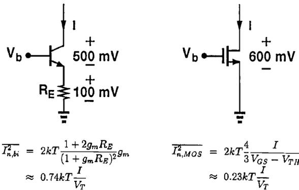
Figure 3: Comparison of noise in bipolar and MOS current sources.
