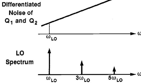
Figure 2: Effect of capacitive degeneration on noise.
