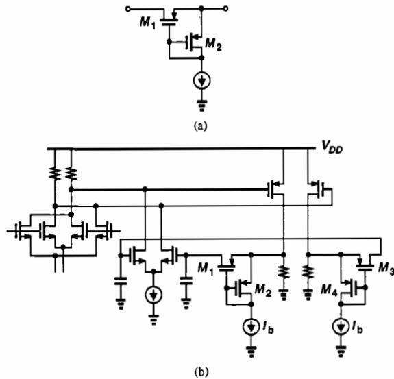
Fig. 9. (a) Floating resistor with controlled gate-source voltage, (b) offset cancellation in the baseband section.
