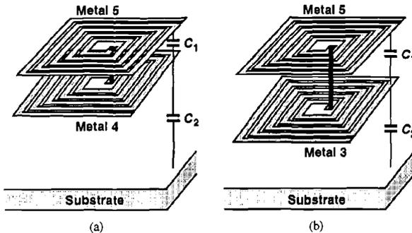
Fig. 6. Two-layer inductor made of (a) metal 5 and metal 4 layers, (b) metal 5 and metal 3 layers.
