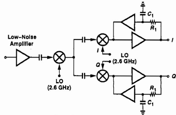
Fig. 1. Receiver architecture.
