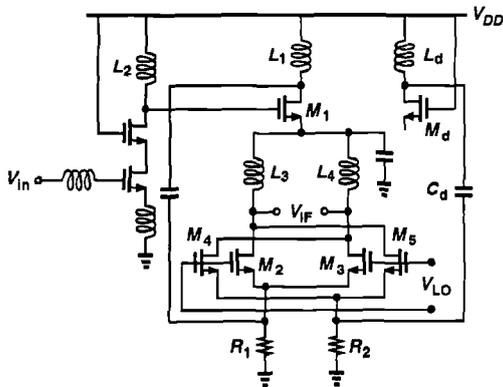
Fig. 5. Cascode LNA followed by stacked double-balanced mixer
