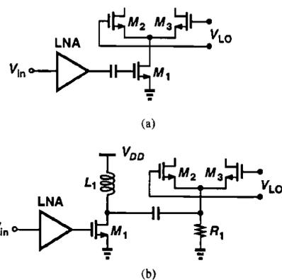
Fig. 3. Removal of flicker noise by capacitive coupling between (a) LNA and mixer. (b) V/I converter and mixer core.
