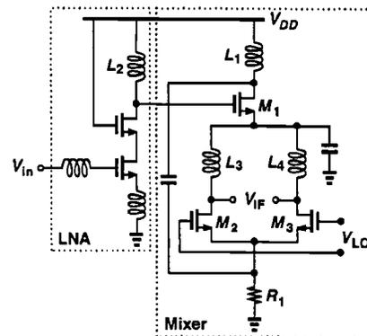
Fig. 4. Cascode LNA followed by stacked single-balanced mixer
