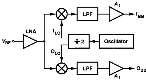
Fig. 1. Receiver architecture.
