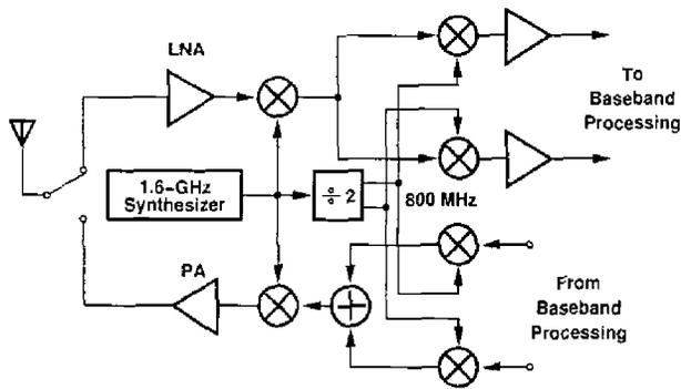
Figure 26.6.1: Transceiver architecture.
