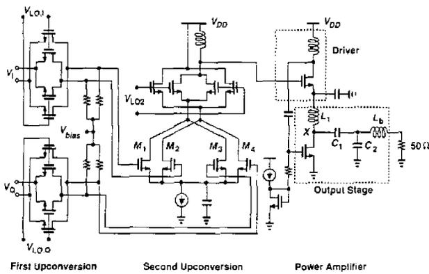
Figure 26.6.3: Transmitter circuit.
