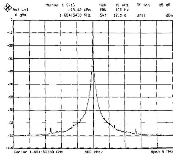
Figure 26.6.7: Synthesizer output spectrum.
