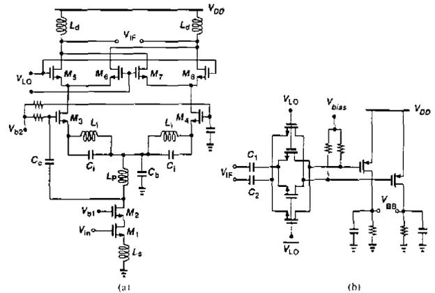
Figure 26.6.2: Receiver circuit (a) RF front-end, (b) IF mixer and amplifiers.
