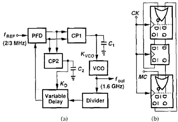
Figure 26.6.4: (a) Synthesizer architecture, (b) divider prescaler.
