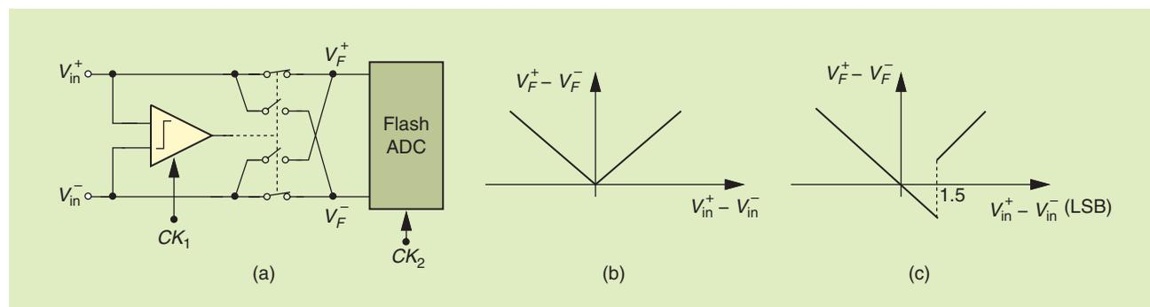
**FIGURE 10:** (a) The flash stage preceded by a polarity detector and (b) the resulting characteristic and the characteristic in the presence of comparator offset.
