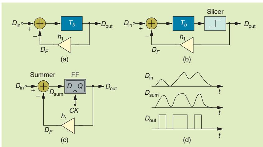
**FIGURE 4:** (a) A feedback loop canceling the first postcursor, (b) the addition of a slicer to suppress amplitude noise, (c) the use of an FF as a delay element and a slicer, and (d) the resulting waveforms.
