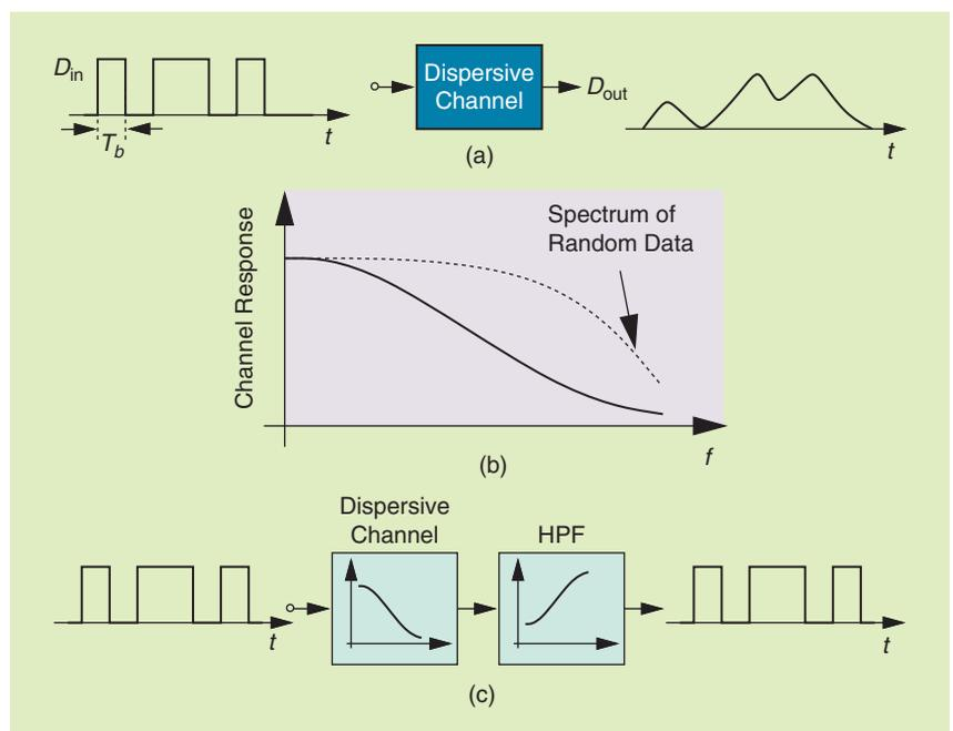
**FIGURE 1:** (a) The dispersion of random data in a lossy channel, (b) the channel frequency response showing attenuation of high-frequency components, and (c) the use of an HPF to equalize the channel.
