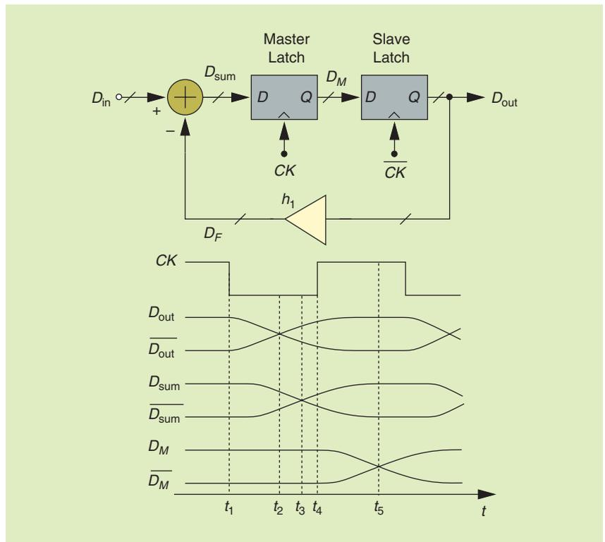
FIGURE 6: A DFE with differential signal paths.
