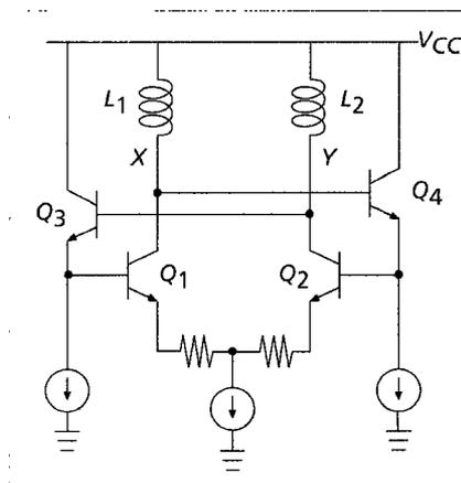
■ **Figure 13.** Bipolar negative- $G_m$  oscillator.
