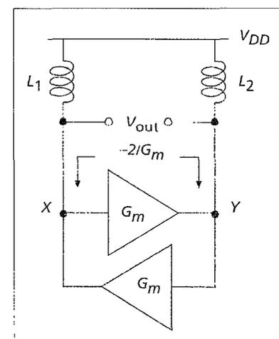
■ **Figure 11.** Oscillator using negative- $G_m$  topology
