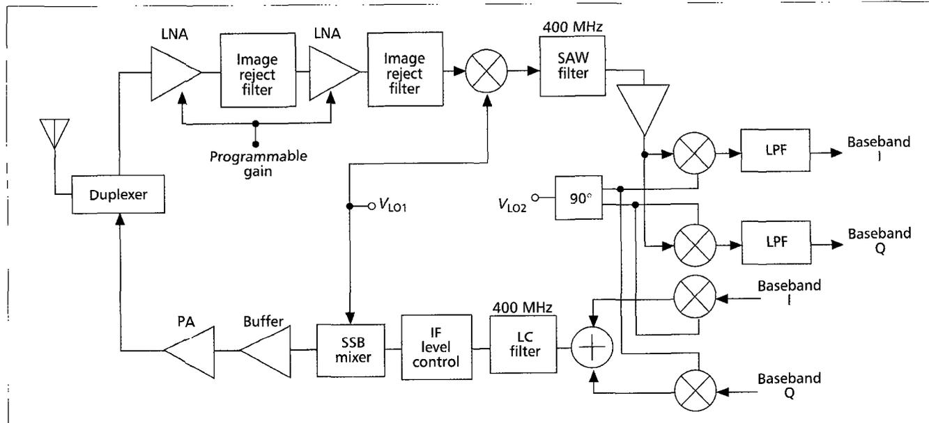
■ Figure 2. The Philips GSM transceiver.
