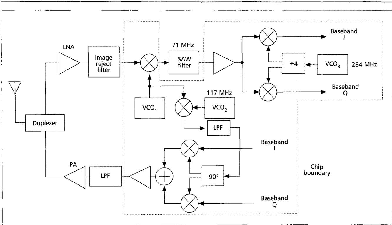
■ Figure 1. Lucent Technologies GSM transceiver.
