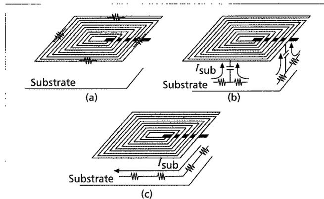
■ **Figure 12** Loss mechanism in monolithic inductors: a) wire resistance; b) electric coupling to substrate; c) magnetic coupling to substrate.
