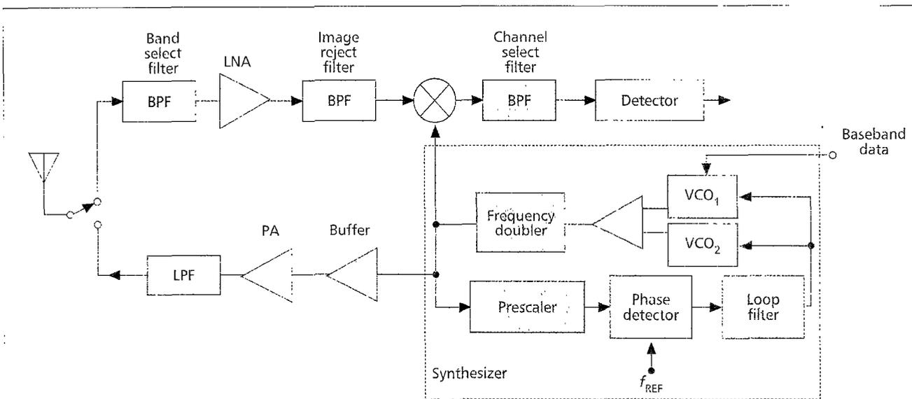
■ Figure 3. Transceiver architecture for digital frequency modulation systems.
