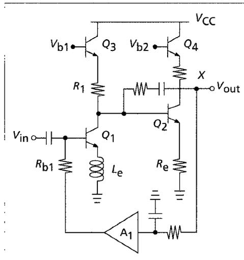
Figure 6. Two-stage bipolar LNA.
