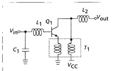
Figure 7. Bipolar LNA using transformer feedback.
