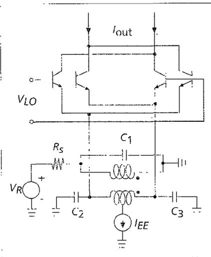
■ **Figure 8.** Double-balanced bipolar mixer with transformer coupling.
