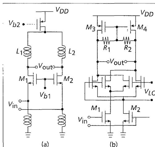
■ **Figure 10.** a) Common-gate CMOS LNA; b) CMOS mixer with grounded-source input pair.
