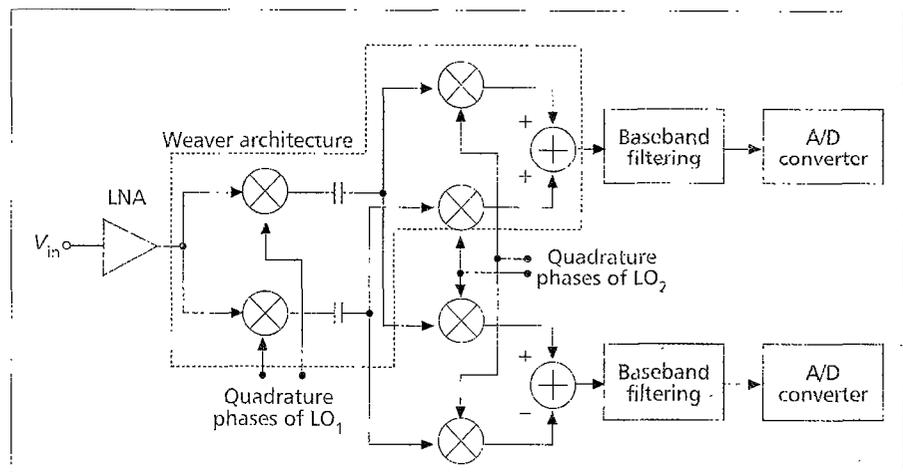
■ Figure 4. The DECT image-reject receiver.
