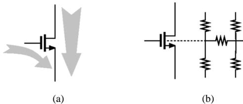
Fig. 19. Illustration of (a) drain noise capacitively coupled to gate and (b) modulation of threshold voltage by body thermal noise.
