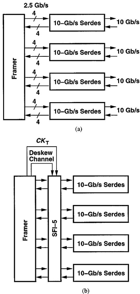
Fig. 11. (a) Interface between a framer and a quad serdes. (b) Addition of SFI-5.
