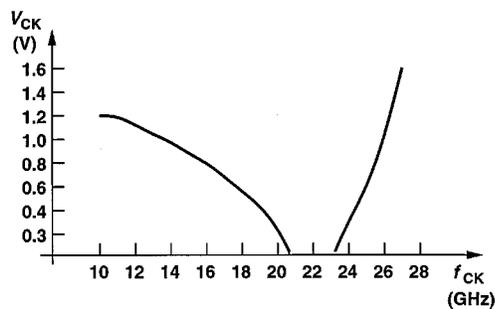
Fig. 3. Divide-by-two circuit sensitivity.
