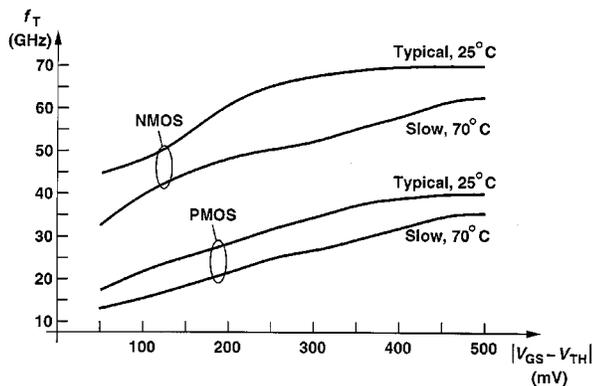
Fig. 2. Transit frequency of 0.13- $\mu\text{m}$  nMOS and pMOS devices.
