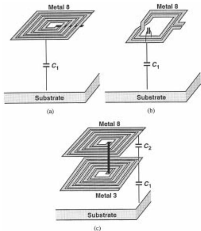
Fig. 4. Spiral inductor structures.
