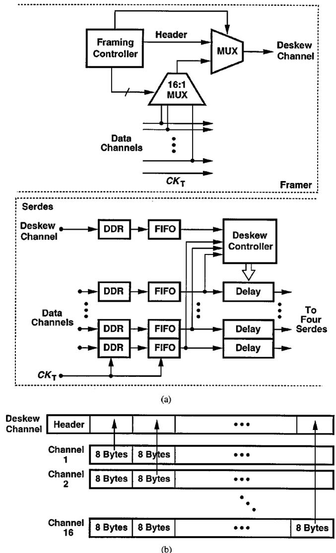
Fig. 12. (a) Details of SFI-5. (b) Deskew frame structure.
