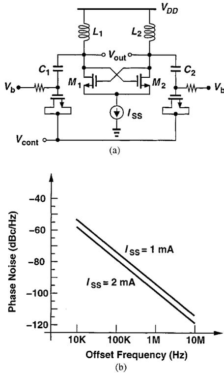
Fig. 19. (a) The 40-GHz LC VCO. (b) Phase noise as a function of frequency offset.
