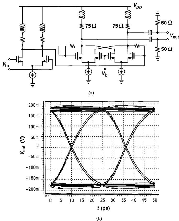
Fig. 18. (a) High-speed output buffer. (b) Simulated output eye diagram.
