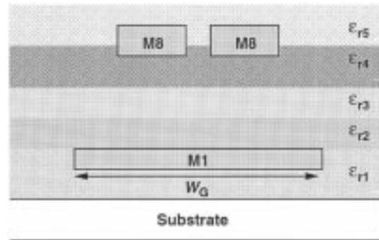
Fig. 9. Actual differential T line in CMOS technology.
