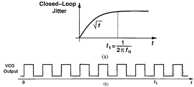
Fig. 20. Accumulation of cycle-to-cycle jitter in a phase-locked oscillator.
