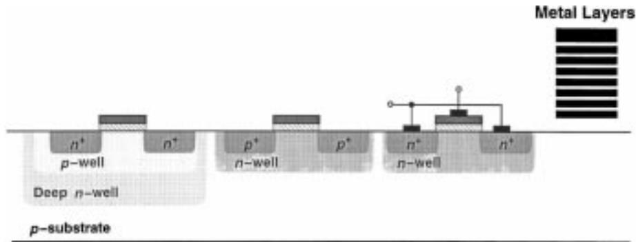
Fig. 1. Typical CMOS process.
