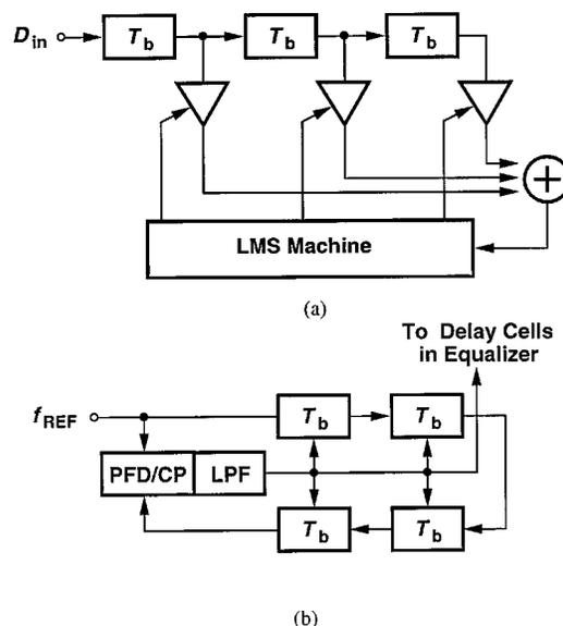
Fig. 15. (a) Tapped delay line equalizer. (b) Use of a DLL to define unit delay.
