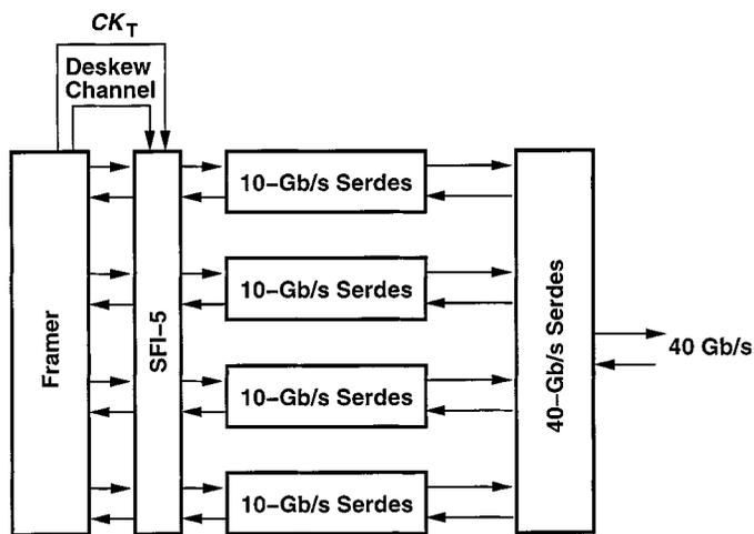
Fig. 13. SFI-5 used in a 40-Gb/s system.
