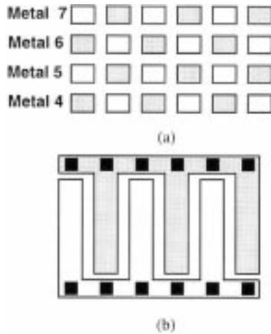
Fig. 8. Fringe capacitor. (a) Side view. (b) Top view.
