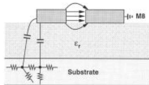
Fig. 7. Coplanar T line.
