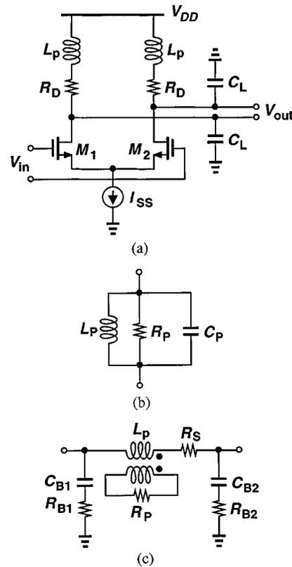
Fig. 16. (a) Inductive peaking. (b) Simple inductor model. (c) More complete inductor model.
