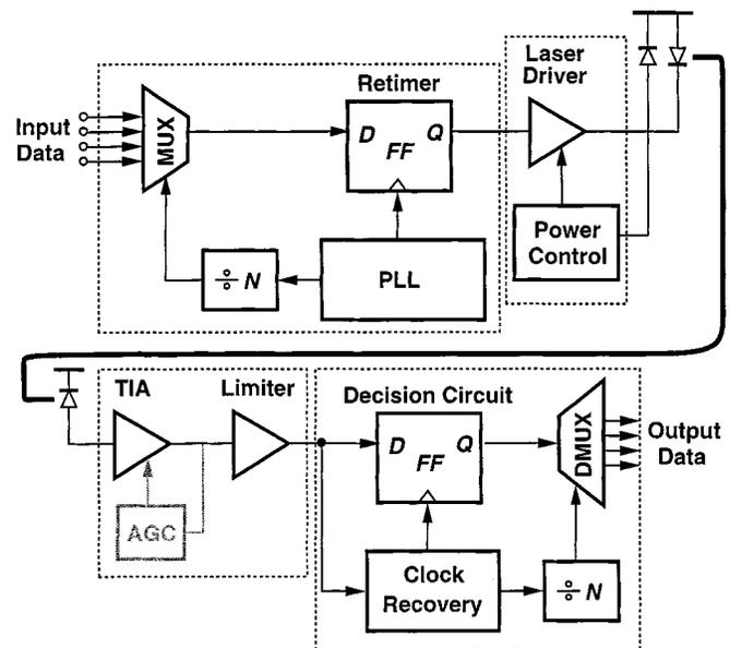
Fig. 10. Traditional OC transceiver.
