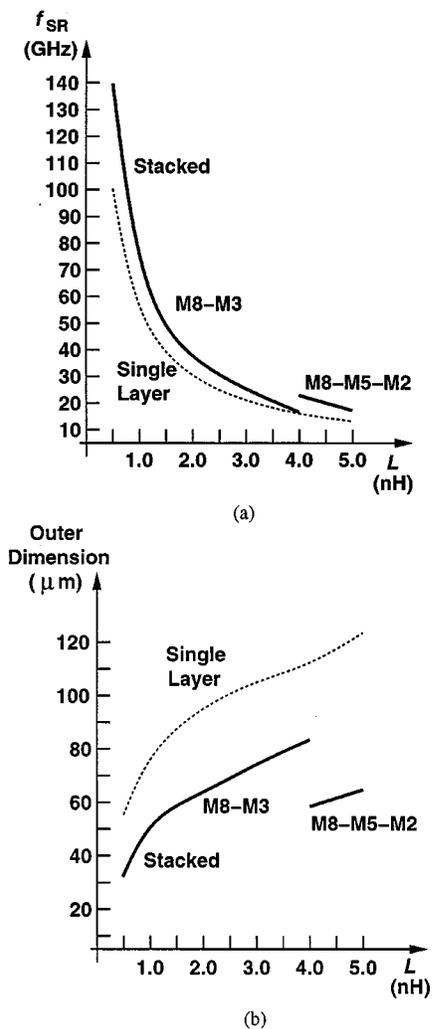
Fig. 5. (a) Self-resonance frequency. (b) Outer dimension of inductors.
