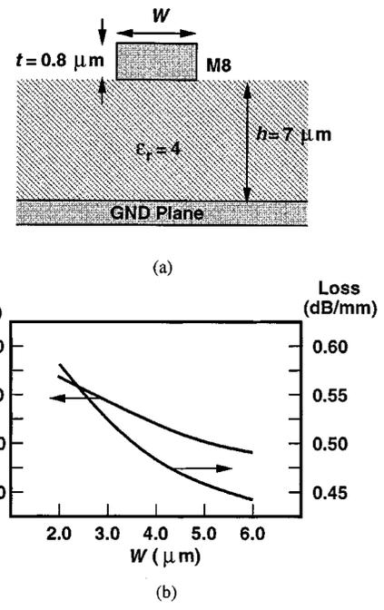
Fig. 6. (a) Microstrip structure in CMOS technology. (b) Loss and characteristic impedance as a function of linewidth.
