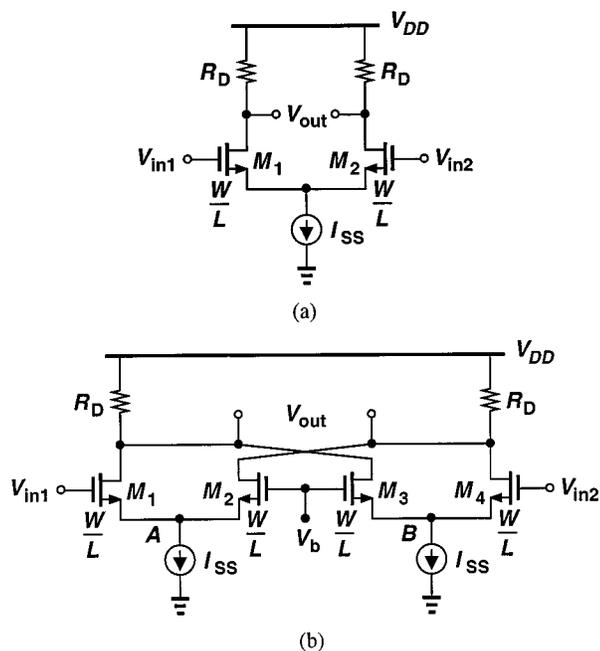
Fig. 17. (a) Simple differential stage. (b)  $f_T$  doubler.
