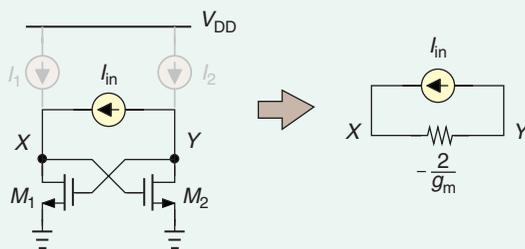
FIGURE 6: The XCP operation from two perspectives.
