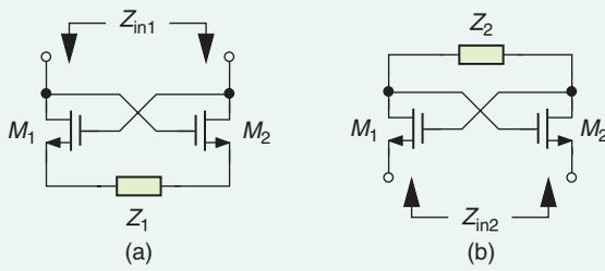
FIGURE 3: An XCP as an impedance negator.
