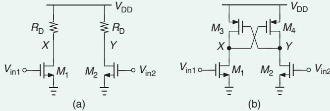
FIGURE 4: A differential buffer using (a) resistive loads and (b) the XCP.
