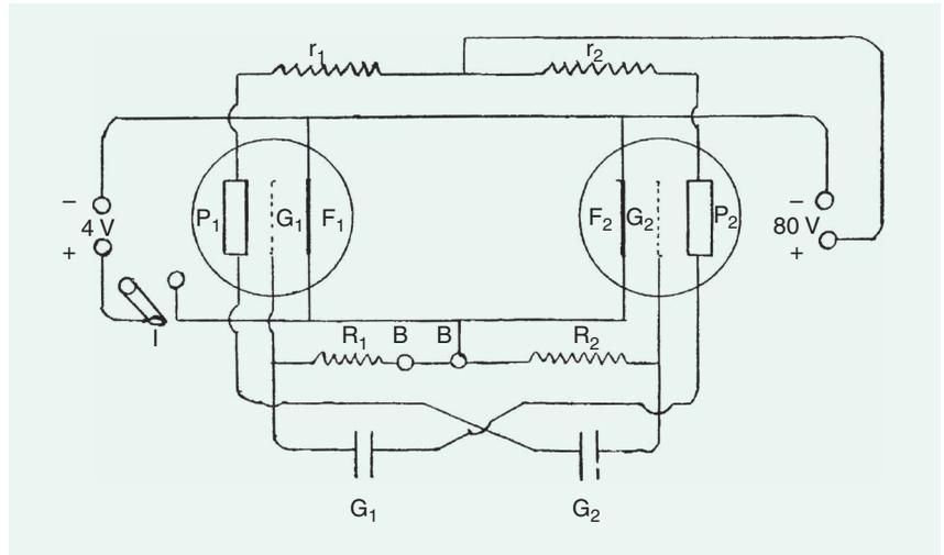
FIGURE 1: A multivibrator using cross-coupled triodes reported in 1919.
