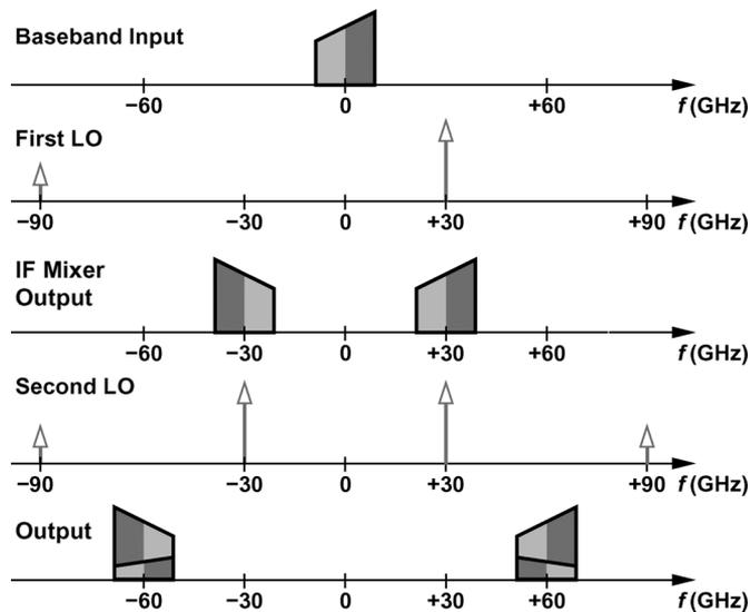
Fig. 3. Half-RF transmitter spectra.
