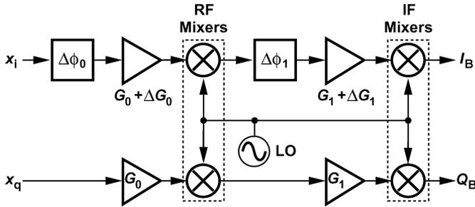
Fig. 24. I/Q mismatch in the receiver.
