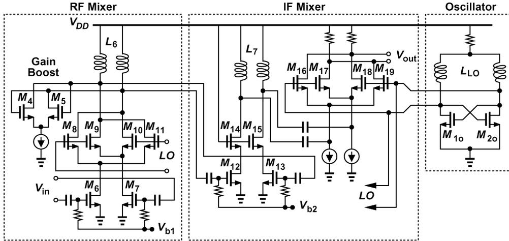
Fig. 11. RF and IF mixers and the oscillator.
