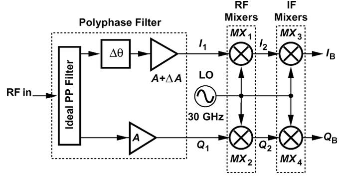
Fig. 7. Gain and phase mismatch in the receiver.
