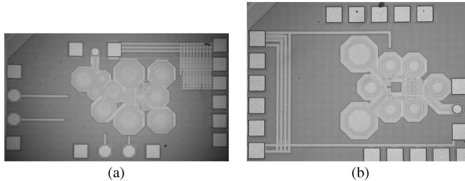
Fig. 18. Die photographs of the receiver and the transmitter.
