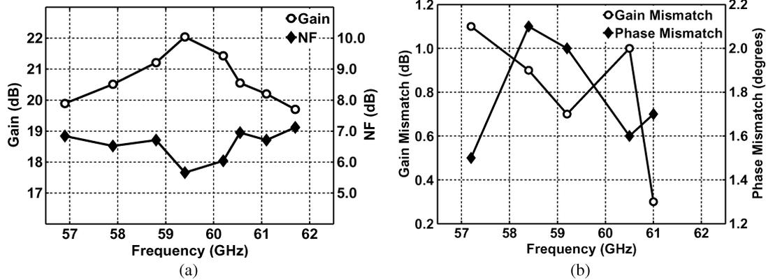
Fig. 19. Measured (a) gain and noise figure, and (b) gain/phase mismatch of the receiver.
