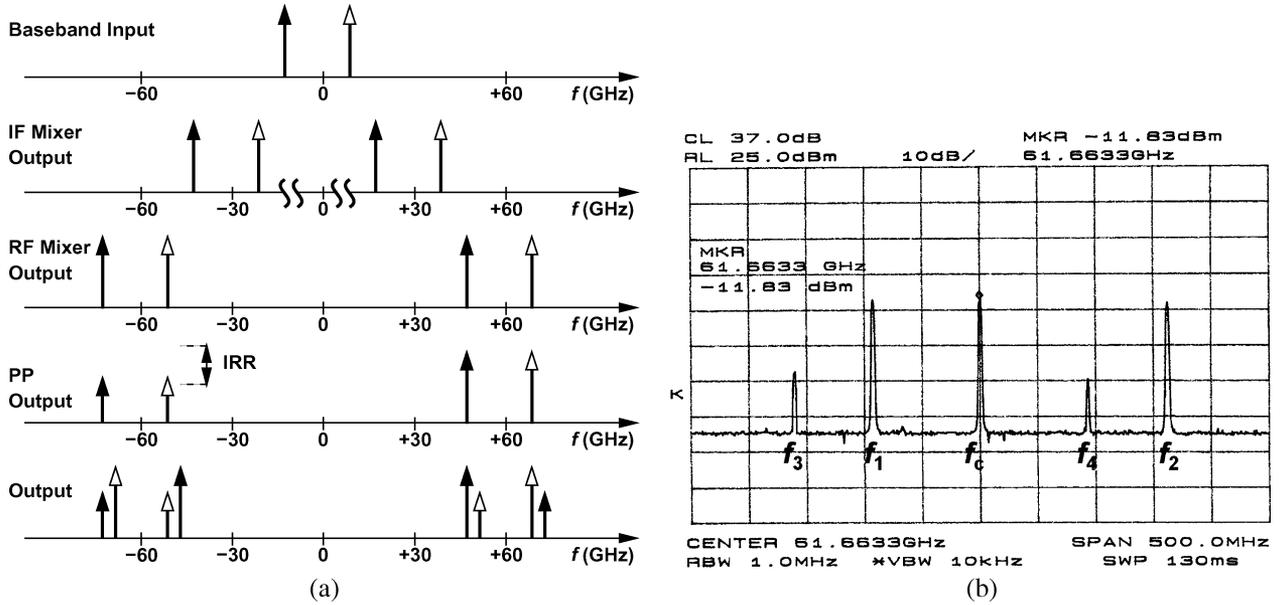
Fig. 21. (a) Asymmetric modulation emulated by two complex tones, (b) measured TX output.
