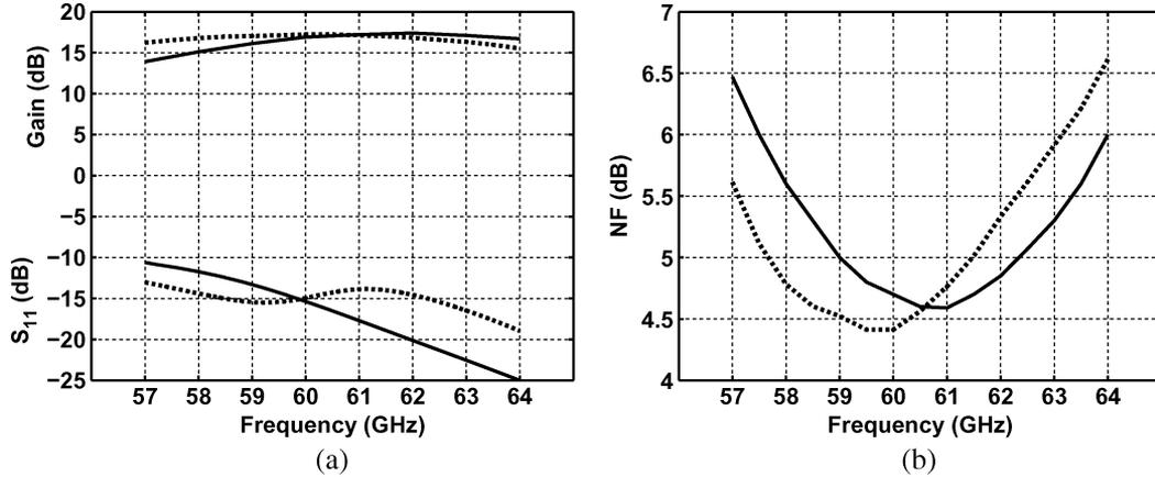
Fig. 13. Simulation of the gain,  $S_{11}$  and NF of the LNA/PPF/mixer cascade with coupling (solid lines) and without (dashed lines).
