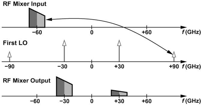
Fig. 5. Elimination of the positive frequency at RF.
