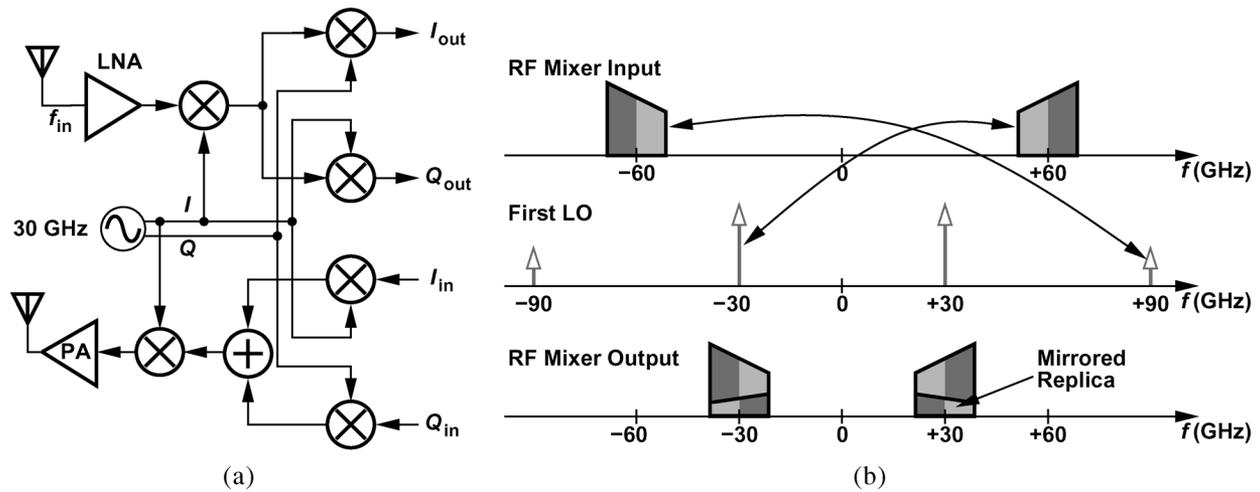
Fig. 2. (a) Half-RF heterodyne transceiver architecture, and (b) receiver spectra.
