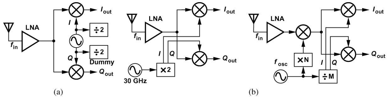
Fig. 1. (a) Generic direct-conversion receiver, (b) direct-conversion receiver with frequency doubler, (c) heterodyne receiver with frequency multiplier and divider.
