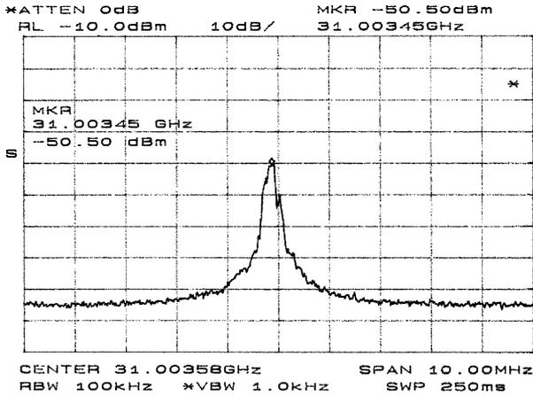
Fig. 23. Measured LO spectrum at TX baseband input.
