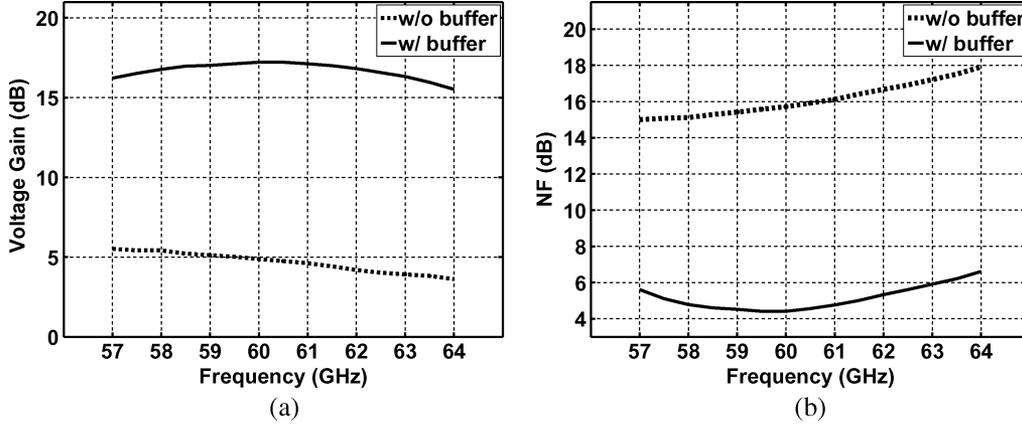
Fig. 10. Simulated (a) gain and (b) noise figure of the LNA/PPF/mixer cascade.
