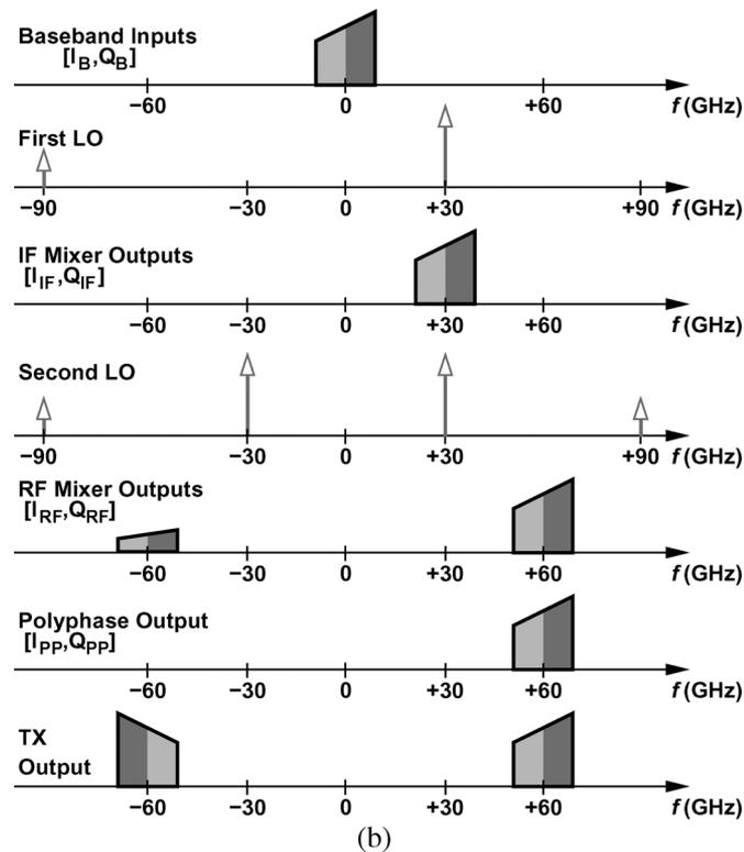
Fig. 14. (a) Transmitter with complex signals. (b) TX spectra.
