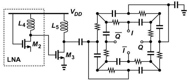
Fig. 9. Schematic of LNA and polyphase filter.
