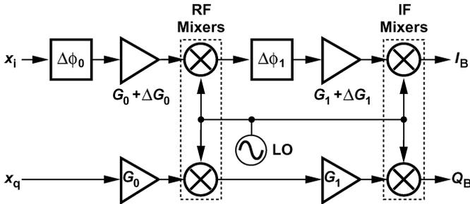
Fig. 24. I/Q mismatch in the receiver.
