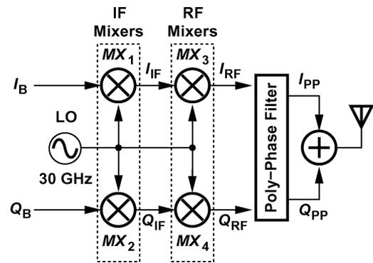
Fig. 15. Architecture of the proposed transmitter.
