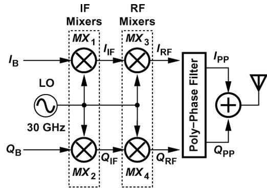
Fig. 15. Architecture of the proposed transmitter.
