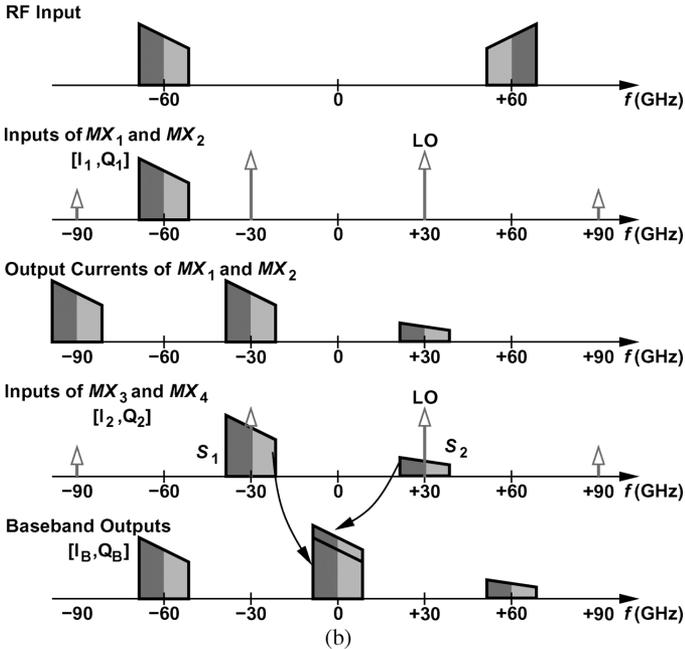
Fig. 6. (a) Proposed half-RF receiver architecture and (b) its spectra.
