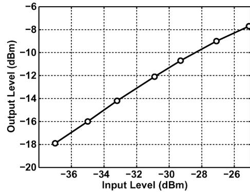
Fig. 20. Measured compression behavior of the receiver.
