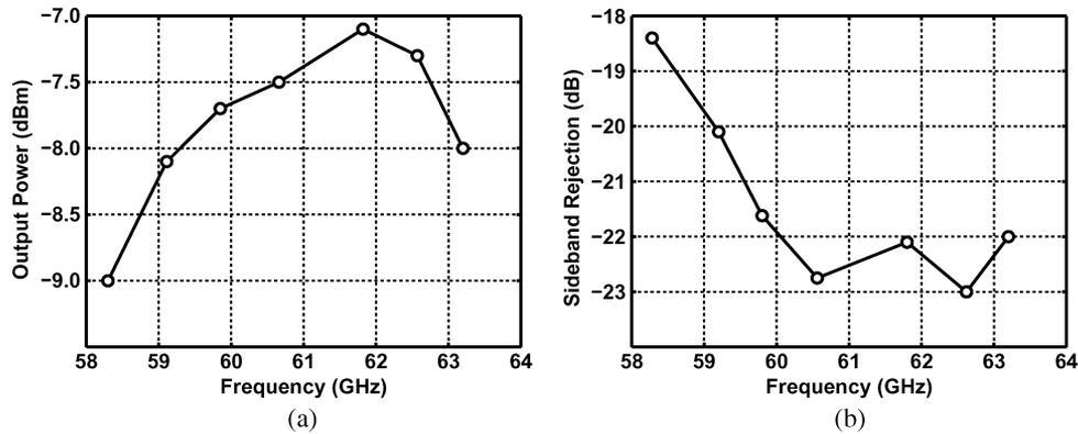
Fig. 22. Measured (a) output level and (b) sideband rejection of the transmitter.
