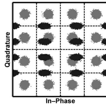
Fig. 4. 16-QAM constellations of ideal and half-RF receivers.
