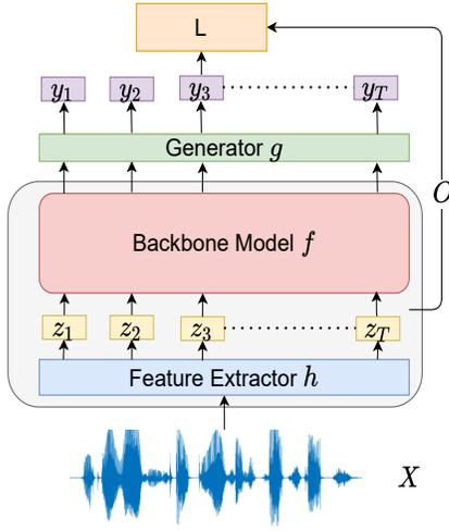
Fig. 1. Proposed self-supervised learning framework.  $h$  is a function to extract speech representation  $Z$ .  $O$  is an operation over  $Z$ .  $f$  is the backbone model for pretraining.  $g$  is a generator that maps the output of the backbone model to have the same dimension as  $O(Z)$  and outputs  $Y$ .  $L$  computes the SSL loss using  $Y$  and  $O(Z)$ .
