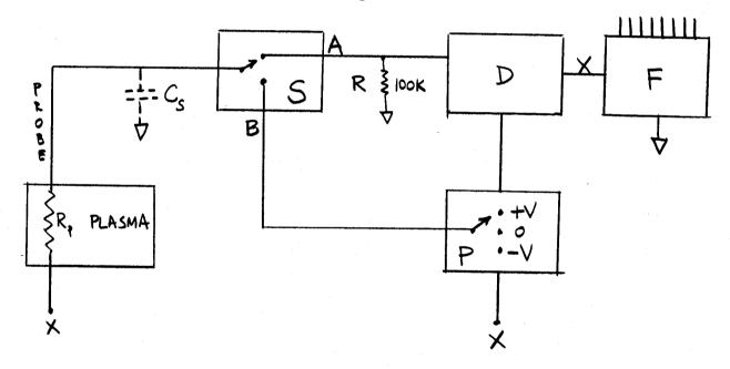
The plasma is represented by a resistance  $R_p \approx 1300~\Omega$ , as found in Sec. 4. The effective plasma capacitance was discussed in Sec. 3 and because of its complexity is omitted here. The stray capacitance  $C_s$  represents the cable between the probe and the electronics. Circuit S is an electric switch which connects the probe alternately to A and B
