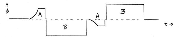
During the interval A in each cycle the probe is connected to a high impedance and rises to the floating potential. If this is found to be positive (negative) relative to a certain reference level, then in interval B the probe is connected to a low-impedance source providing a negative (positive) potential, thus reducing (increasing) the electron flux collected by the probe and thus pulsing the plasma potential back toward the reference level.
