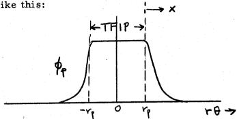
The potential  $\phi_p$  in the TFIP will fall off to the surrounding potential (taken here to be 0) in a sheath of thickness =  $O(\lambda_D)$ . If, for instance,  $\phi_p$  is positive, there will be an excess of electrons in the sheath and an equal excess of ions in the TFIP. To bring  $\phi$  up to  $\phi_p$ , a negative charge must be removed from the TFIP; we compute this by computing the negative charge in the sheath.
