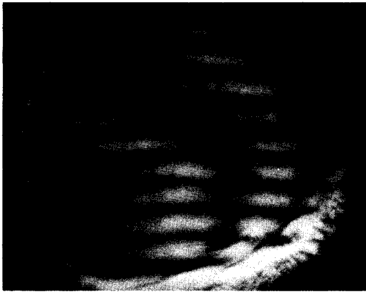
FIG. 4. Radial ruby interferogram from which the density scalelength was measured. The magnetic field is parallel to the fringes.
