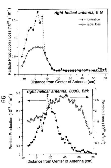
Helicon discharge operated with 15 mTorr of Ar gas, 2.0 kW of 27.12 MHz RF power, and various axial magnetic fields.
