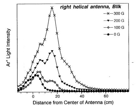
The profiles for magnetic fields from 0 to 900 G, at intervals of 100 G, reveal that the second (helicon) peak increases in magnitude but remains fixed in position. The emission profiles are very asymmetric with respect to the center of the antenna, suggesting preferential plasma production in the direction of the magnetic field for this antenna helicity.
