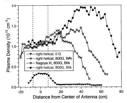
The axial density variation can be shown to follow from pressure balance. In steady state, the z component of the electron equation of motion is:
