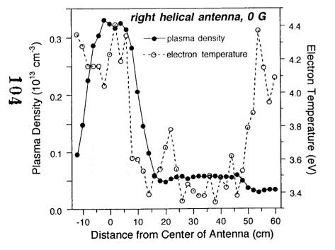
In the helicon mode with  $B/\!/k$  the electron temperature peaks 16 cm from the center of the antenna and cools downstream; the electron density is uniform within the antenna region and increases by a factor of two several antenna lengths (50 cm) downstream.
