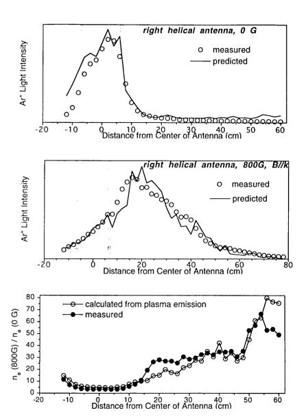
The dependence of plasma production on the magnetic field's direction was investigated. When two opposite field directions were used, the plasma emission peaks away from the antenna, in the direction of the magnetic field.
