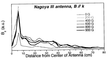
As was the case for the plasma emission and plasma density measurements, the standing wave pattern measured depends on the direction of the axial magnetic field. These patterns confirm that at these power levels helical antennas efficiently excite the m=+1 azimuthal helicon mode but fail to couple to the m=-1 mode.
