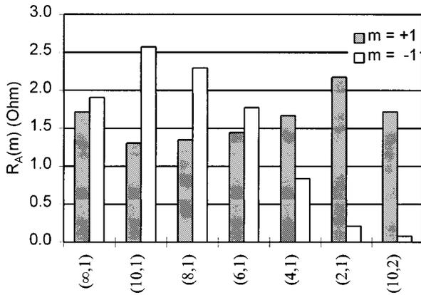
FIG. 13. The dependence of antenna plasma resistance on density profile  $(s,t)$  and wave polarization for  $m = \pm 1$  shown for progressively more peaked density profiles.
