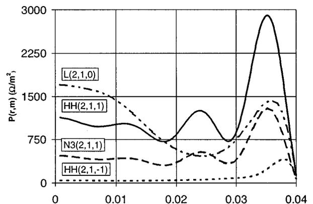
FIG. 16. Dependence of power absorption  $P(r,m)$  on antenna configuration and wave polarization for a parabolic density profile.
