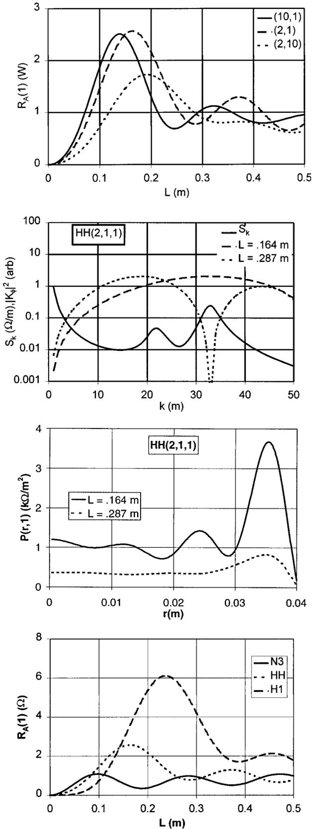
FIG. 21. (a) Plasma resistance as a function of antenna length for an HH antenna and plasmas with various density profiles  $(s,t)$ . (b) specific power density  $S_k$  and antenna power spectrum for the optimal  $L_{opt}=0.164$  m, and first minimal  $L_{m1}=0.287$  m, antenna lengths of (a), and (c) power deposition profile for antenna lengths of (b). Variation of antenna plasma resistance with antenna length for three antennas (d).
