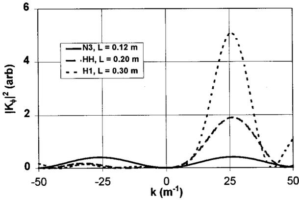
FIG. 3. Power spectrum (arbitrary units) for the  $m=1$  component of three antennas. Positive  $k$  corresponds to the direction of  $\mathbf{B}_0$ .
