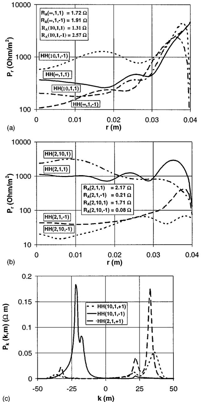
FIG. 14. The dependence of power absorption  $P(r,1)$  on density profile for (a) two near uniform profiles, (b) two axially peaked profiles, and (c) spectral antenna plasma resistance for HH(10,1,+1), HH(10,1,-1), and HH(2,1,+1).
