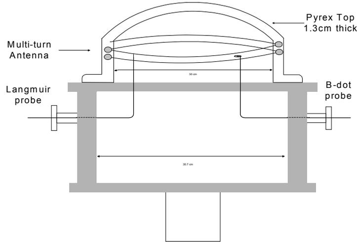
Fig. 1. Schematic diagram of the experimental setup, including antenna, dogleg Langmuir and  $B_z$ -dot probes. Probe heights and antenna locations are arranged so that profiles are obtained in the plane of the antenna. Typical operating parameters are:  $N_p \sim 5 \cdot 10^{10} - 5 \cdot 10^{11} \text{ cm}^{-3}$ ,  $P_{RF} \leq 400 \text{ W}$ ,  $T_e \sim 2-4 \text{ eV}$ ,  $P_O = 1-20 \text{ mT}$ ,  $f_{RF} \sim 2-7 \text{ MHz}$ .
