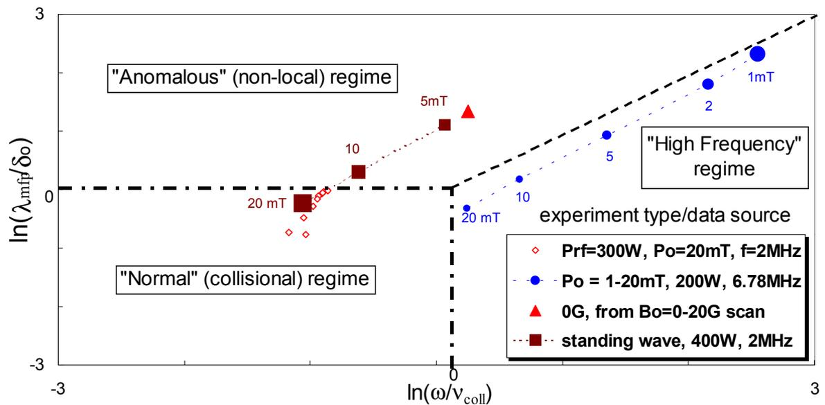
Fig. 7. Collisional regimes in parameter space for each experiment: ASE non-locality parameter  $\ln(\lambda_{mfp}/\delta_0)$  vs  $\ln(\omega/v_{coll})$ , where  $\delta_0 \equiv (c/\omega_{pe}) \cdot (1 + v_{coll}^2/\omega^2)^{1/4}$  and  $v_{coll} \equiv$  electron collisional frequency ( $\equiv v_{en}$  in these discharges).
