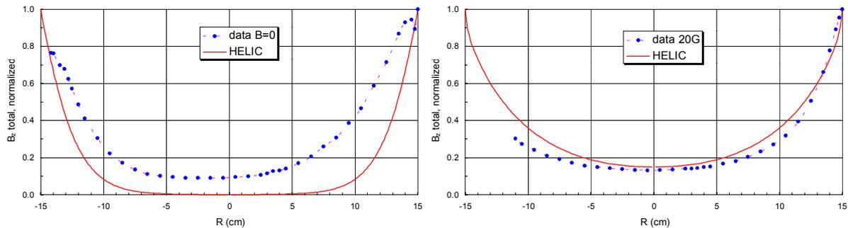
Fig. 6. Comparison of RF field penetration in an unmagnetized (left) and weakly-magnetized (right,  $B_0=20\text{G}$ ) ICP, otherwise operating in the anomalous regime (2MHz, 5mT). Anomalous field penetration appears to be suppressed by application of a static  $\mathbf{B}_0$ -field, as shown by agreement between the 20G data and HELIC curves.
