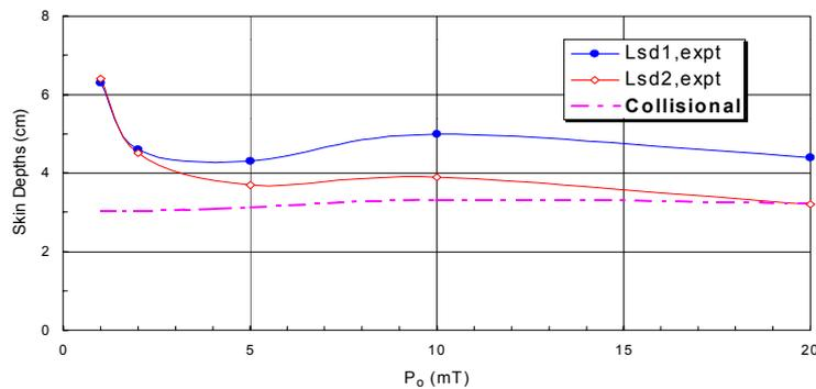
Fig. 3. Comparison between experimental  $L_{sd}$ ’s and collisional theory (pink).  $200 \text{ W}$ ,  $6.78 \text{ MHz}$ ,  $P_O = 1-20 \text{ mT}$ .
