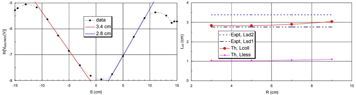
Fig. 2. Semi-log plots of  $B_z$ -dot profile (left) in “normal” collisional regime ( $300 \text{ W}$ ,  $2 \text{ MHz}$ ,  $20 \text{ mT}$ ). Edge features (“wings”) are probably due to the effects of induced currents in nearby conductors. Least squares fits yield experimental  $L_{sd}$ ’s (right, dashes), in good agreement with collisional theory ( $L_{coll}$ , red).
