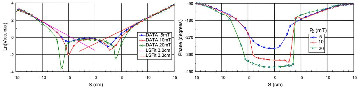
Fig. 4.  $\text{Ln}(B_z\text{-dot})$  amplitude (left) and phase (right) radial profiles, for  $P_o = 5\text{-}20\text{ mT}$ ,  $400\text{W}$ ,  $2\text{MHz}$ . Local minima (nodes) and  $\sim 180^\circ$  phase “jumps” at  $|s|\sim 5\text{cm}$  are indications of interference and/or standing-wave-like behavior. These effects become more apparent as  $P_o$  ( $v_{en}$ ) increases, in apparent contradiction to ASE theory.
