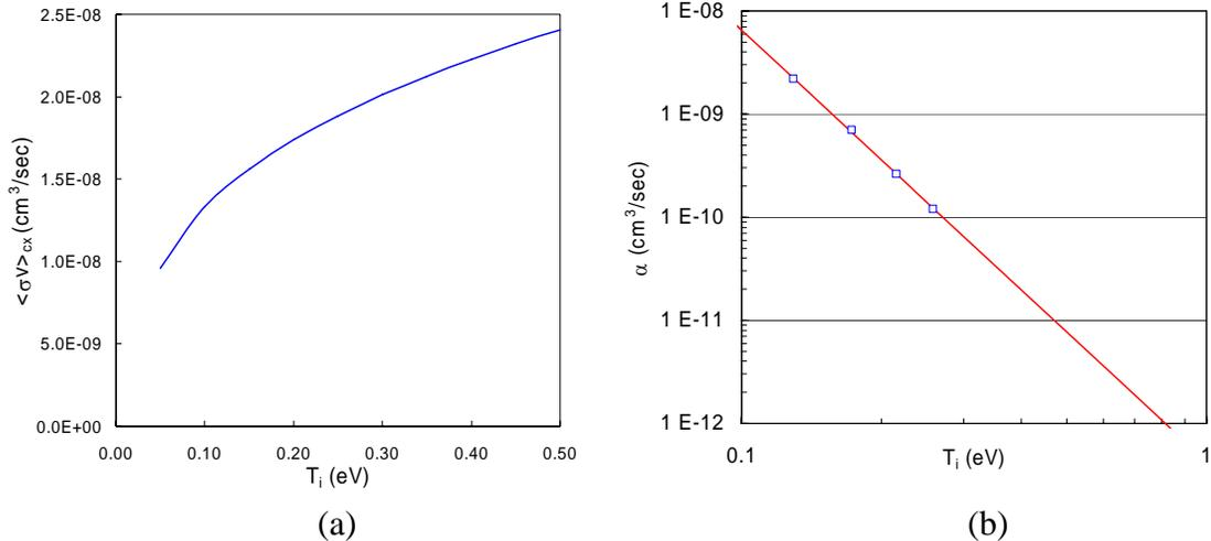
Fig. 1. (a) Ion-neutral collision probability and (b) recombination coefficient vs. lithium ion temperature.
