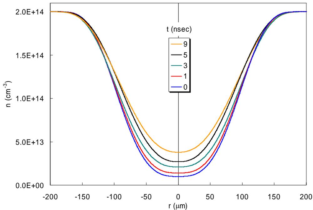
Fig. 6. Diffusion of a profile with  $r_0 = 200 \mu\text{m}$ ,  $f = 0.05$ ,  $s = 3$ ,  $t = 6$ , and  $n_0 = 2 \times 10^{14} \text{cm}^{-3}$ .
