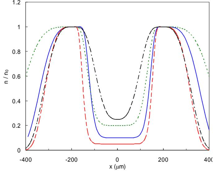
Fig. 2. Hollow density profiles obtainable by varying the parameters  $f$ ,  $s$ ,  $t$ ,  $u$ ,  $v$ , and  $w$  for  $r_0 = 200 \mu\text{m}$
