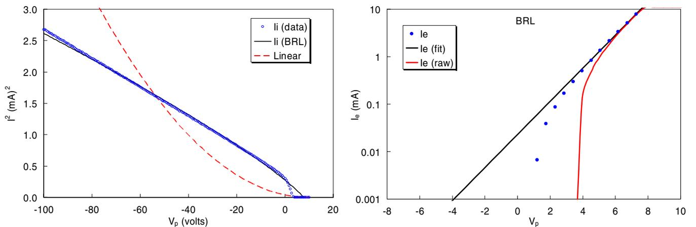
Figure 6. Ion and electron fits using the BRL theory. The dashed line (- - -) is for  $I_i \propto (V_s - V_p)$ .
