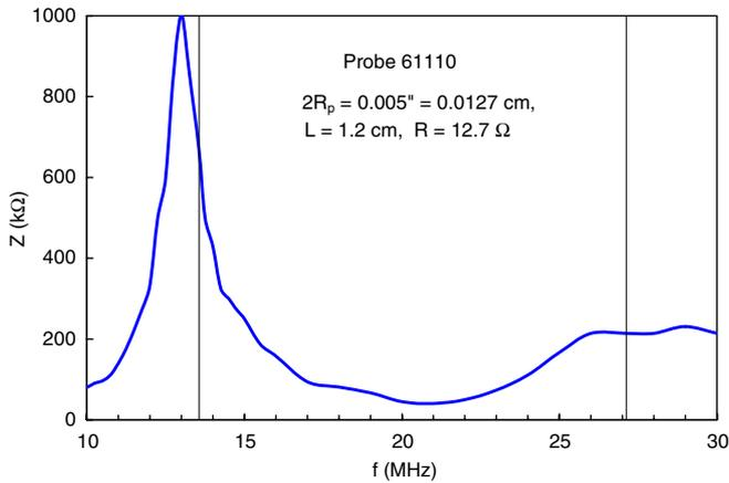
**Figure 8.** Impedance characteristic of a sample probe. The vertical lines mark 13.56 and 27.12 MHz.
