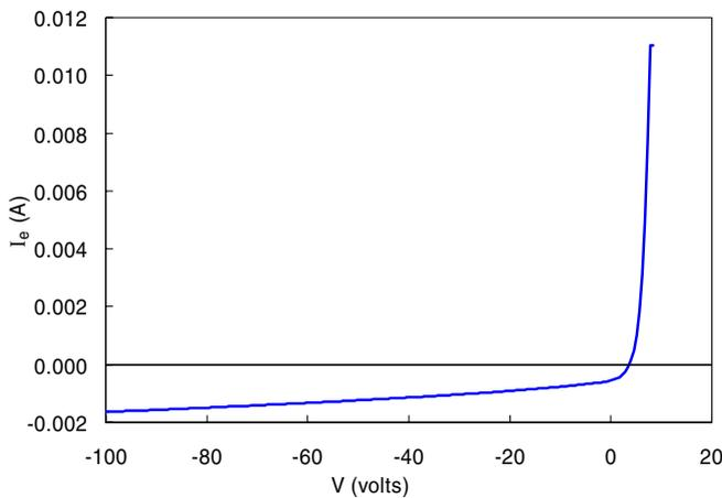
**Figure 2.** A sample  $I$ - $V$  curve from an RF plasma.
