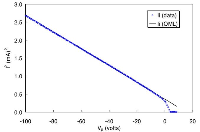
**Figure 3.** Measured ion current squared (O) and an OML fit (—) from  $-100$  to  $-10 \text{ V}$ . Here  $I^2$  is actually the total probe current  $I_p^2$ , cut off at  $V_f$ .
