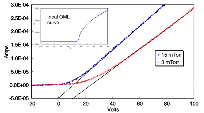
**Figure 15.** Example of potential pulling by saturation electron current.
