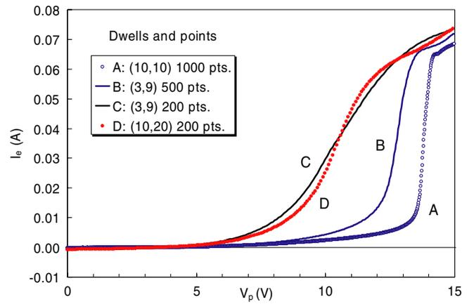
**Figure 9.** Dwell test with a 5 mil probe at X1, Z2,  $y = 0$  in 15 mTorr of Ar at 2400 W.
