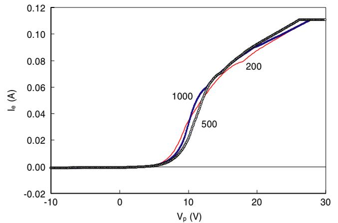
**Figure 10.** Dwell test varying only the number of points in a sweep.
