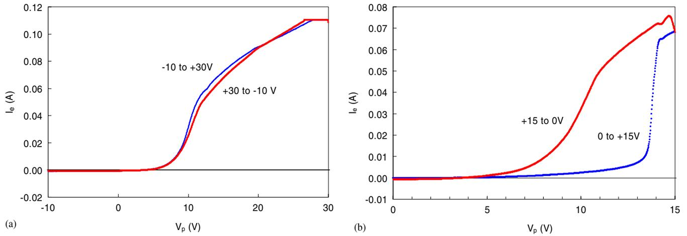
**Figure 12.**  $I$ - $V$  curves taken forward and backward with a 5 mil probe at X1, Z2,  $y = 0$ , 15 mTorr, 2400 W, 1000 points, dwells (3, 9) in (a) and (10, 10) in (b).
