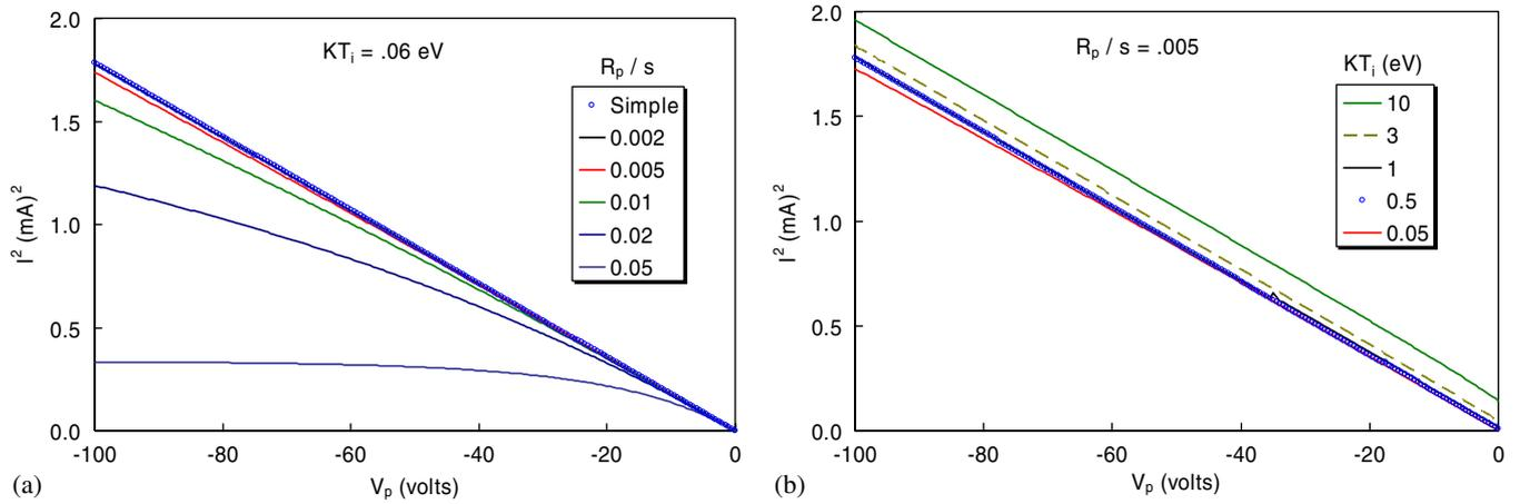
**Figure 16.** (a) Exact OML curves for various  $\varepsilon$  with  $T_i = T_n$ . The approximate OML formula is shown by the points (O). (b) Variation of exact OML curves with  $T_i$  for  $\varepsilon = 0.005$ . In each case, the order of the curves follows that in the legend.
