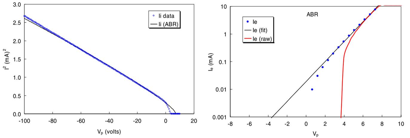
Figure 5. Ion and electron fits using the ABR theory.
