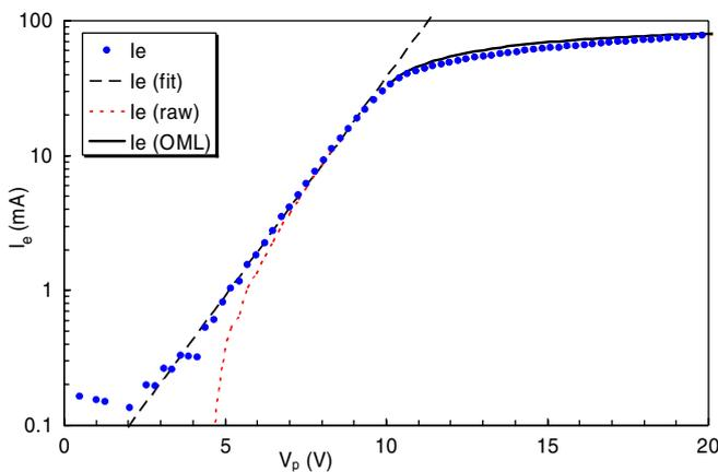
**Figure 19.** Example of OML fit (—) to electron saturation current (●).
