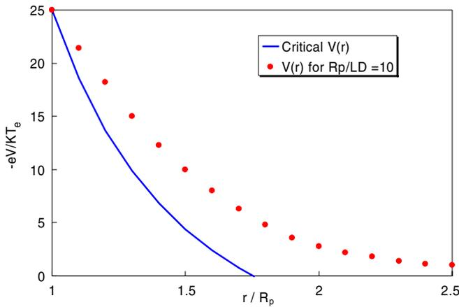
**Figure 18.** Critical  $V(r)$  for OML validity (—) compared with a computed profile (●) for BRL theory.
