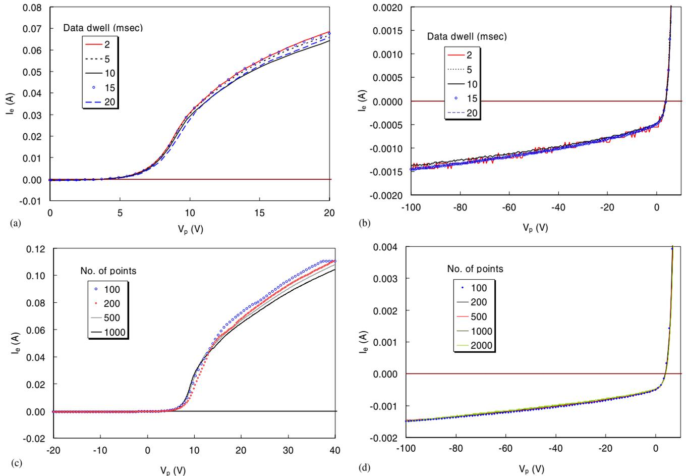
**Figure 11.** Dwell test with a 3 mil probe at X2, Z2,  $y = 0$  in 15 mTorr of Ar at 2400 W: (a)  $-100$  to  $+20$  V, 200 points, start dwell 3 ms, electron part; (b) same, ion part; (c)  $-20$  to  $+40$  V, dwells (3, 9); (d) same,  $-100$  to  $+10$  V.
