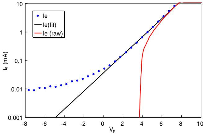
**Figure 4.** Semilog plot of negative probe current  $-I_p$  versus probe voltage before (—) and after (●) subtraction of the ion current, as fitted by OML theory.
