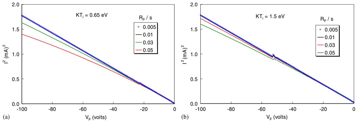
**Figure 17.** Exact OML curves for various  $\varepsilon$  with (a)  $KT_i = 0.65$  eV; (b)  $KT_i = 1.5$  eV. The kink in the curves is caused by switching to the asymptotic formula for  $\text{erfc}(x)$  when  $e^\eta$  is large enough to cause numerical overflow.
