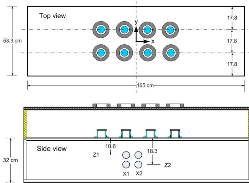
**Figure 1.** Top and side views of the plasma source.
