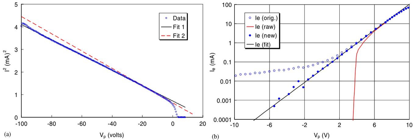
**Figure 14.** (a) Fits to the ion data over different ranges. (b) Electron current as corrected with ion Fit 2.
