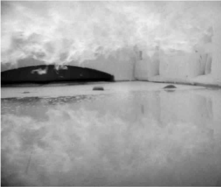
**Fig. 16.3** Photographs of the combustion space and the surface of the glassmelt in glass melting furnaces, transverse flames with batch logs, secondary foams, and free melt surface. Reproduced by permission of Research Association of the German Glass Industry (HVG) © 2010.
